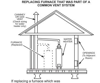
commonly vented with another gas appliance, the size of the existing vent pipe for that gas appliance must be checked. Without the heat of the original furnace flue products, the existing vent pipe is probably oversized for the single water heater or other appliance. The vent should be checked for proper draw with the remaining appliance.
