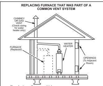
If replacing a furnace which was commonly vented with another gas appliance, the size of the existing vent pipe for that gas appliance must be checked. Without the heat of the original furnace flue products, the existing vent pipe is probably oversized for the single water heater or other appliance. The vent should be checked for proper draw with the remaining appliance.
