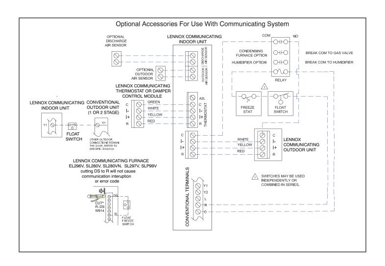
**TABLE 13**Field Wiring Applications With Conventional Thermostat
