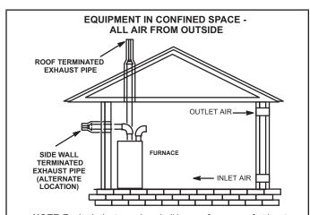
NOTE-Each air duct opening shall have a free area of at least one square inch per 2,000 Btu (645mm² per .59kW) per hour of the total input rating of all equipment in the enclosure. If the equipment room is located against an outside wall and the air openings communicate directly with the outdoors, each opening shall have a free area of at least 1 square inch per 4,000 Btu (645mm² per 1.17kW) per hour of the total input rating of all other equipment in the enclosure.
