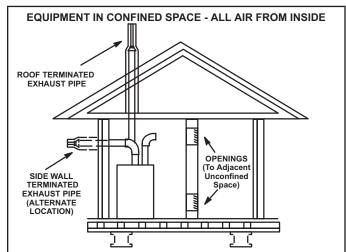
**NOTE** - Each opening shall have a free area of at least one square inch per 1,000 Btu (645mm<sup>2</sup> per .29kW) per hour of the total input rating of all equipment in the enclosure, but not less than 100 square inches (64516mm.<sup>2)</sup>.
