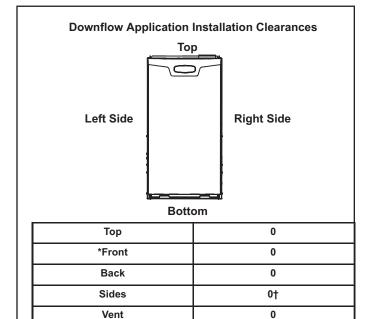
\*Front clearance in alcove installation must be 24 in. (610 mm). Maintain a minimum of 24 in. (610 mm) for front service access. †Allow proper clearances to accommodate condensate trap and vent pipe installation.
