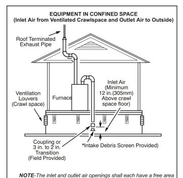
of at least one square inch per 4,000 Btu (645mm² per 1.17kW) per hour of the total input rating of all equipment in the enclosure.
