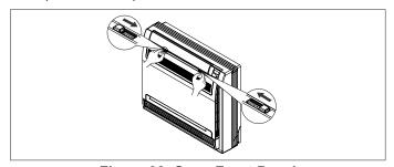
Figure 32. Open Front Panel
