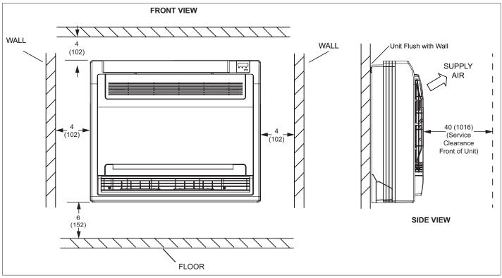
Figure 6. Indoor Unit Clearances - Inches (mm)
