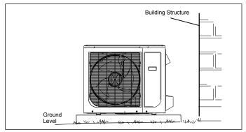
Figure 8. Install Unit Level
