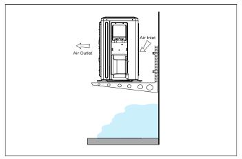
Figure 10. Outdoor Unit on Brackets above Snow Line
