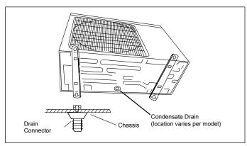
Figure 16. Condensate Drain
