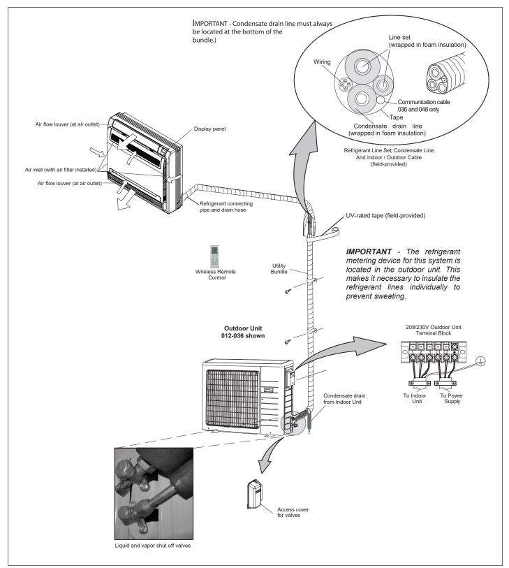
Figure 1. Typical System Shown
