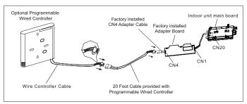
Figure 34. Connecting Optional Programmable Wired Controller
