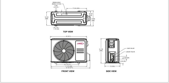
Figure 3. MLB012S4S Outdoor Unit Dimensions - Inches (mm)
