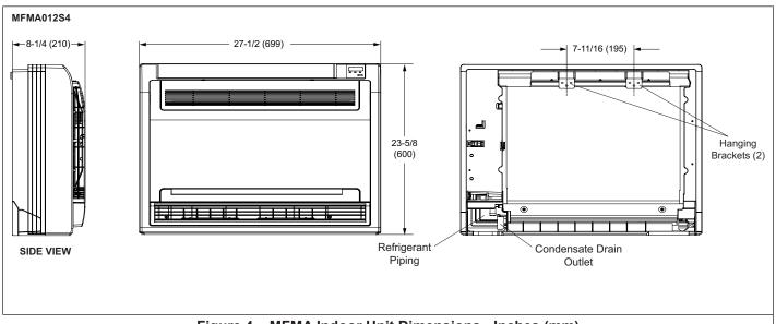
Figure 4. MFMA Indoor Unit Dimensions - Inches (mm)
