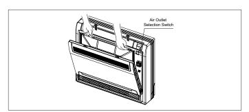
Figure 33. Open Front Panel
