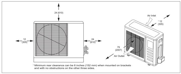
Figure 5. Outdoor Unit Clearances - Inches (mm)
