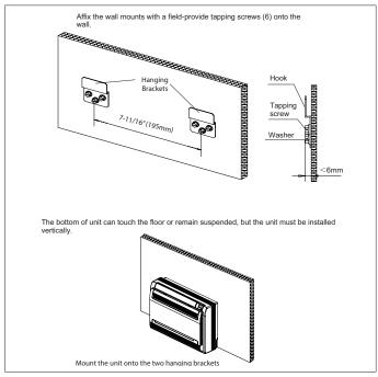
Figure 7. Mounting Unit to Wall
