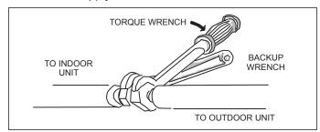
Figure 22. Tighten Flare Nut
