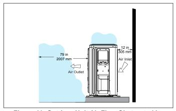
Figure 11. Outdoor Unit Air Flow Obstructed by Snow
