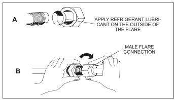
Figure 21. Making Connections (Male to Female Connection)
