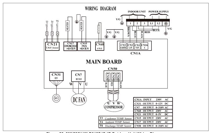
Figure 26. 208/230V MLB012S4S-\*P Outdoor Unit Wiring Diagram
