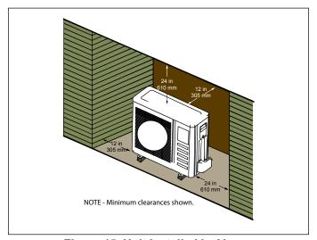
Figure 15. Unit installed in Alcove
