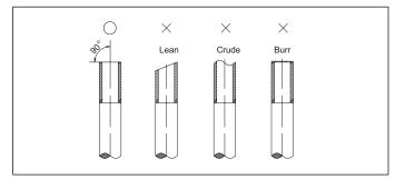
Figure 20. Cutting Pipe
