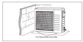
Figure 17. Securing Outdoor Unit to Slab
