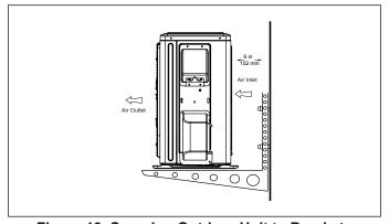
Figure 19. Securing Outdoor Unit to Brackets
