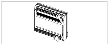
Figure 31. Airflow Adjustment - Left and Right
