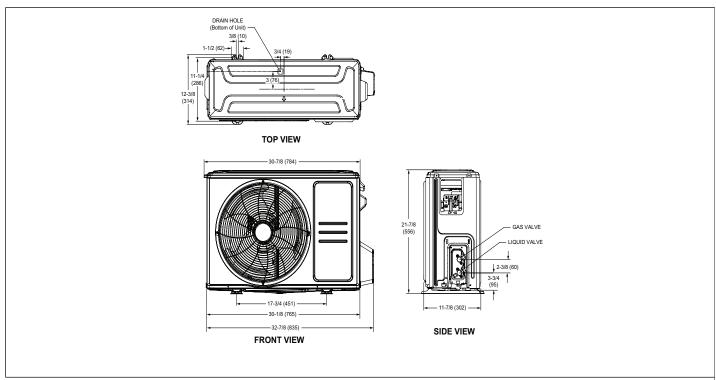
Figure 2. 208/230V - MPC012S4S Outdoor Unit Dimensions - Inches (mm)
