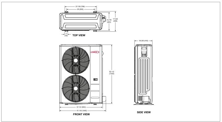
Figure 5. MPC048S4S-\*P- Unit Dimensions - inches (mm)
