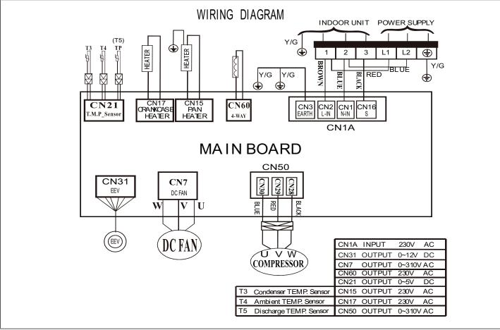
Figure 42. 208/230V MPC009S4S-\*P Outdoor Unit Wiring Diagram
