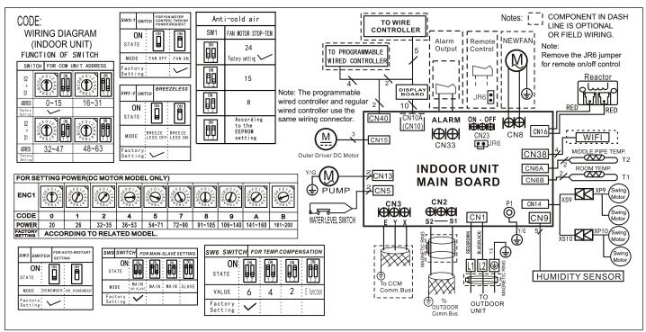
Figure 41. M33C Unit Wiring Diagram (All Sizes)
