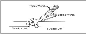
Figure 37. Tighten Flare Nut
