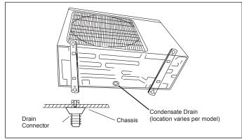
Figure 31. Condensate Drain
