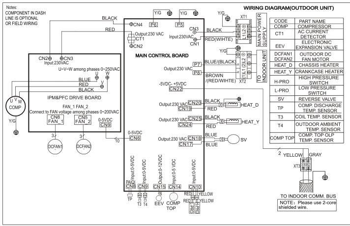
Figure 47. 208/230V MPC048S4S-\*P Outdoor Unit Wiring Diagram
