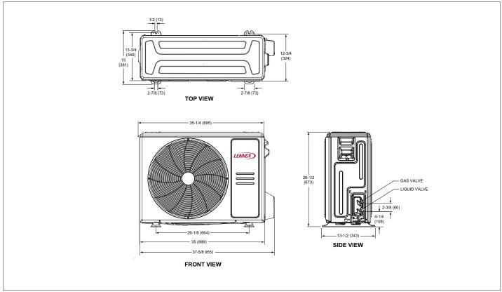
Figure 3. MPC018S4S-\*P - Unit Dimensions - inches (mm)
