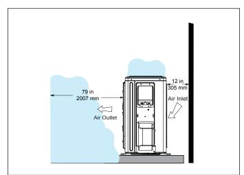
Figure 26. Outdoor Unit Air Flow Obstructed by Snow
