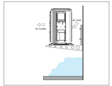
Figure 25. Outdoor Unit on Brackets above Snow Line
