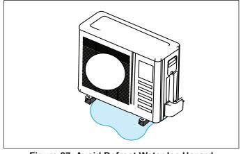
Figure 27. Avoid Defrost Water Ice Hazard
