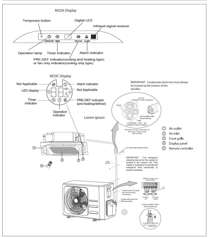
Figure 1. Typical M33C Single Zone System Shown
