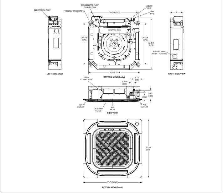
Figure 11. M33C Indoor Cassette Unit Dimensions - inches (mm)
