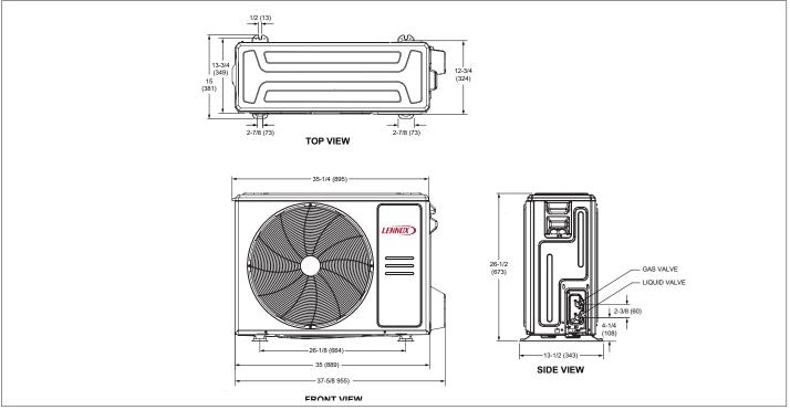
Figure 7. MLB018S4S-\*P - Unit Dimensions - inches (mm)
