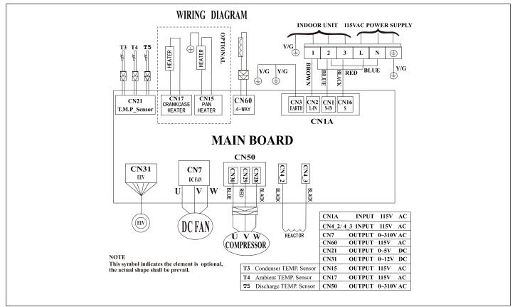
Figure 43. 208/230V MPC012S4S-\*P Outdoor Unit Wiring Diagram
