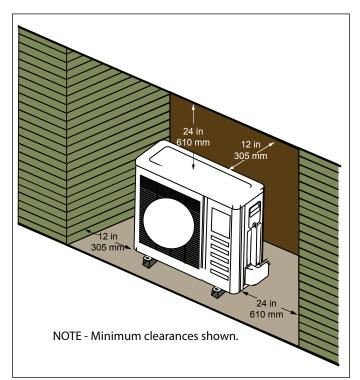
Figure 30. Unit installed in Alcove
