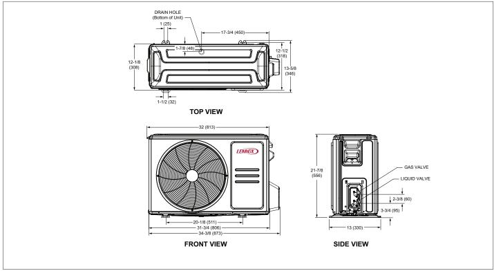
Figure 6. MLB009S4S-\*P and MLB012S4S-\*P - Unit Dimensions - inches (mm)
