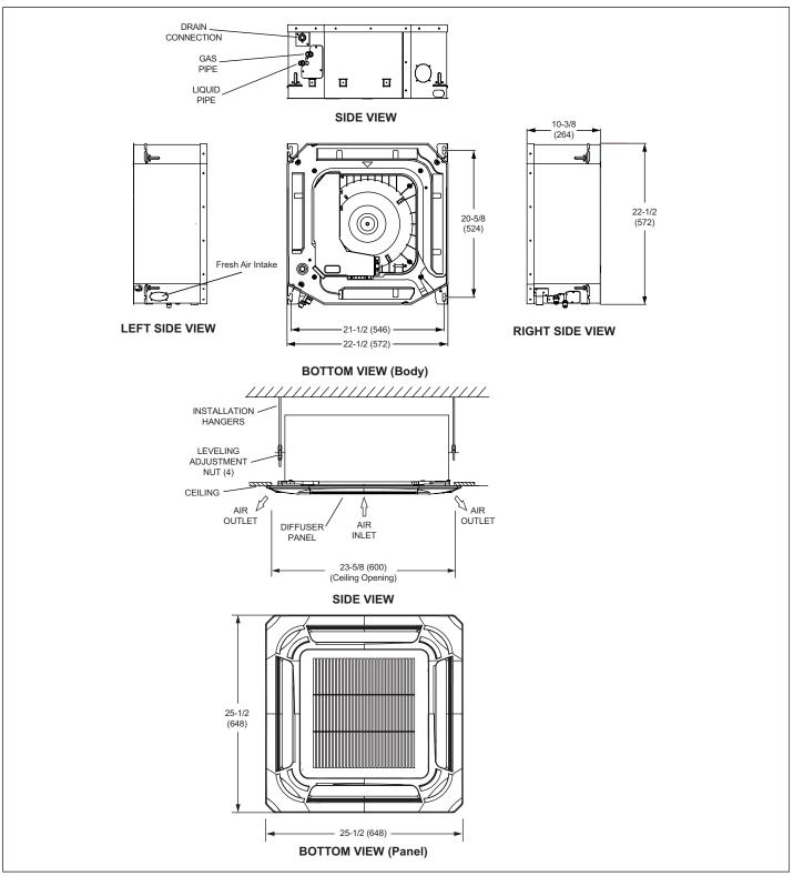
Figure 10. M22A Indoor Cassette Unit Dimensions - inches (mm)
