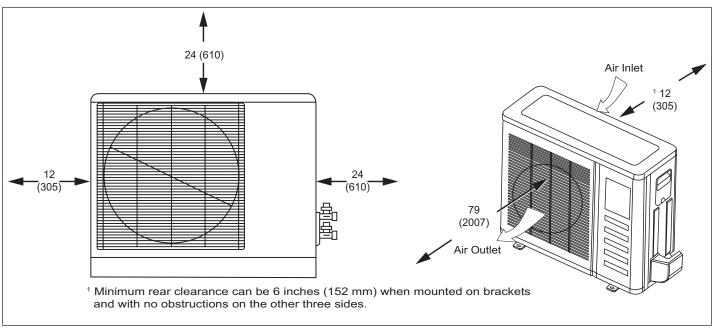
Figure 12. Outdoor Unit Clearances - inches (mm)
