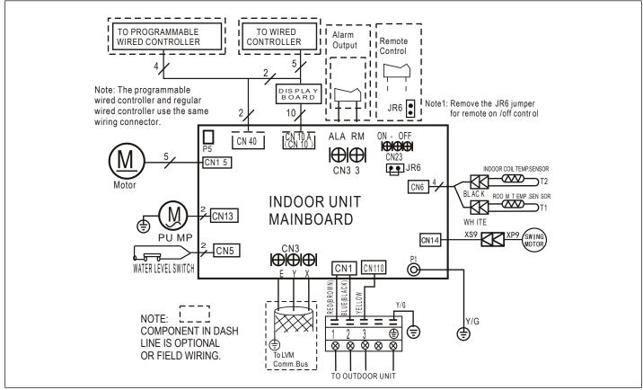
Figure 40. M22A009S4-\*P, M22A012S4-\*P and M22A018S4-\*P Unit Wiring Diagram
