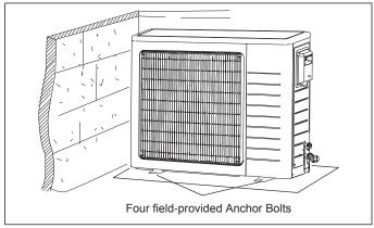
Figure 32. Securing Outdoor Unit to Slab
