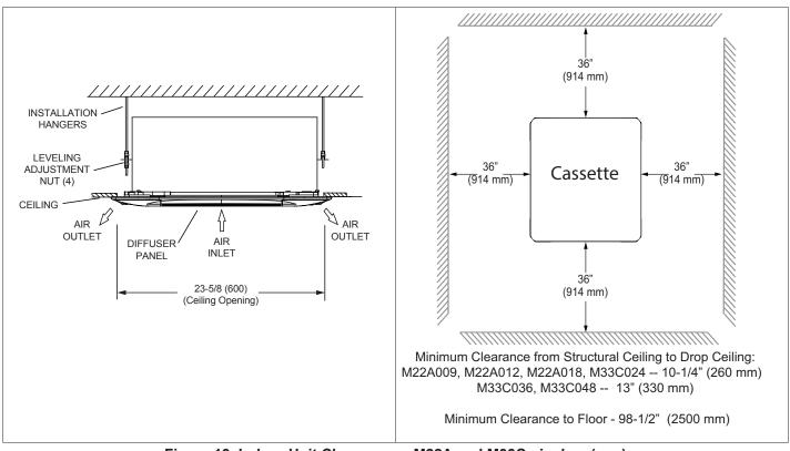
Figure 13. Indoor Unit Clearances - M22A and M33C - inches (mm)
