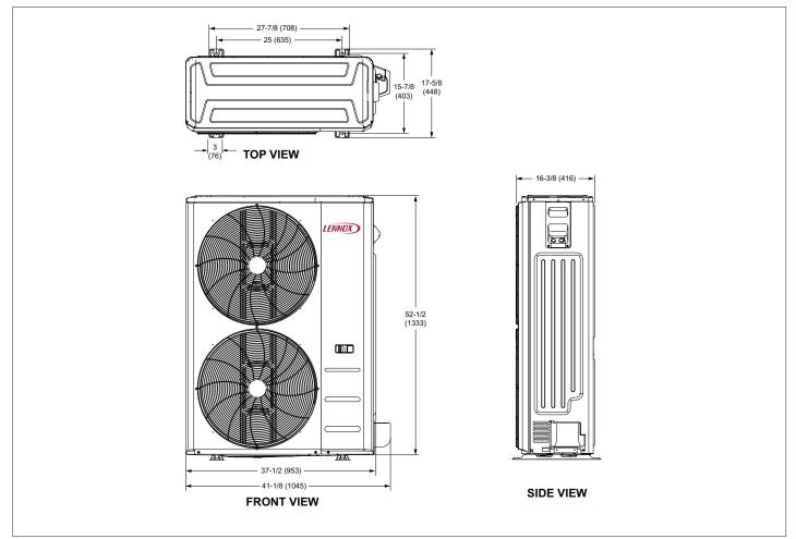
Figure 9. MLB036S4S-\*P and MLB048S4S-\*P- Unit Dimensions - inches (mm)
