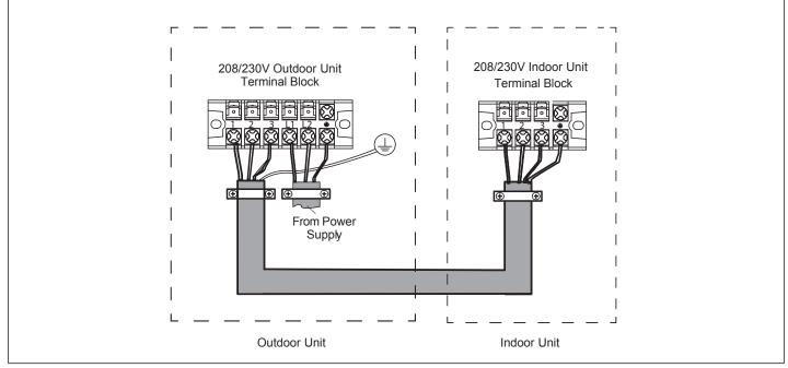
Figure 38. Single Zone Wiring (09K to 24K)
