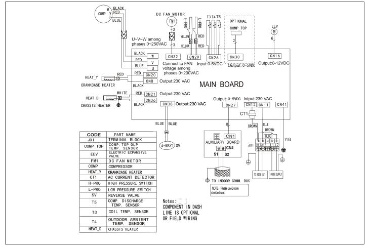
Figure 46. 208/230V MPC036S4S-\*P Outdoor Unit Wiring Diagram
