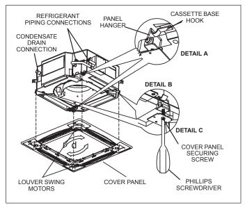
Figure 18. Install Cover Panel
