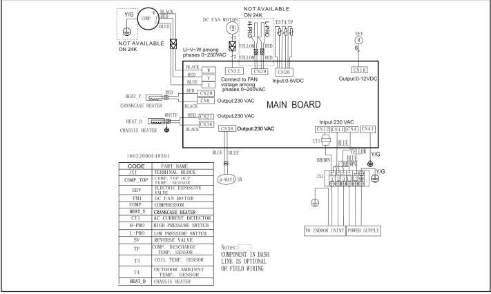
Figure 50. 208/230V MLB024S4S-\*P Outdoor Unit Wiring Diagram
