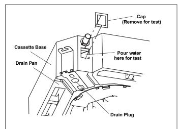
Figure 21. Test Condensate Drain
