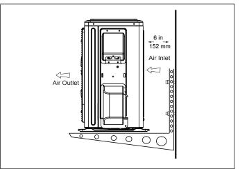
Figure 34. Securing Outdoor Unit to Brackets
