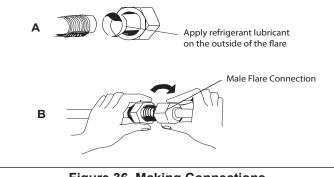
Figure 36. Making Connections (Male to Female Connection)
