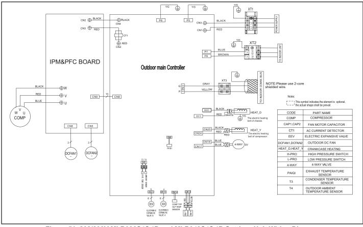
Figure 51. 208/230V MLB036S4S-\*P and MLB048S4S-\*P Outdoor Unit Wiring Diagram
