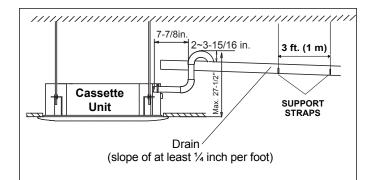
Figure 22. Indoor Unit Condensate Drain
