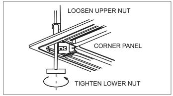
Figure 20. Adjust Unit Height through Corner Panel
