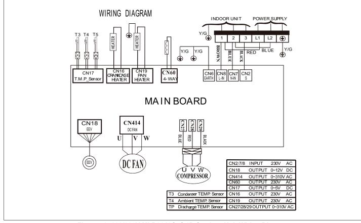
Figure 49. 208/230V MLB0018S4S-\*P Outdoor Unit Wiring Diagram
