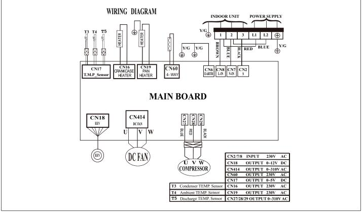
Figure 44. 208/230V MPC018S4S-\*P Outdoor Unit Wiring Diagram
