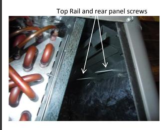
Fig. 8: Screw Top Rail to rear panel
