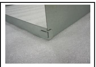
Fig. 6a: Tab Inside Support with Top Rail
