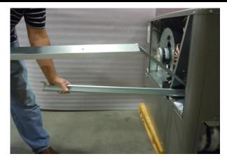
Fig. 7a: Scissor 3-piece assembly into unit
