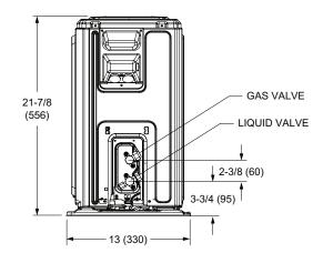
**FRONT VIEW**NOTE – Due to Lennox' ongoing commitment to quality, Specifications, Ratings, and Dimensions are subject to change without notice and without incurring liability. Improper installation, adjustment, alteration, service or maintenance can cause property damage or personal injury. Installation and service must be performed by a qualified installer and servicing agency.
