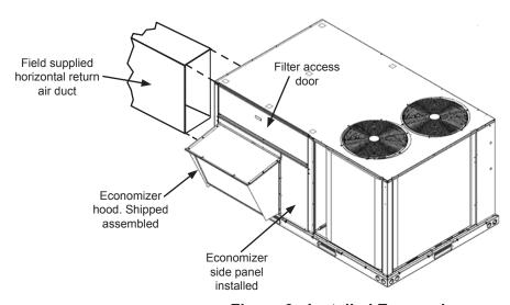
Figure 6 - Installed Economizer
