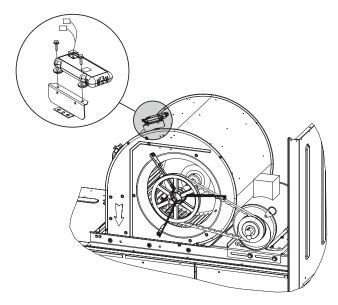
Figure 10 - Mixed Air Sensor Location
