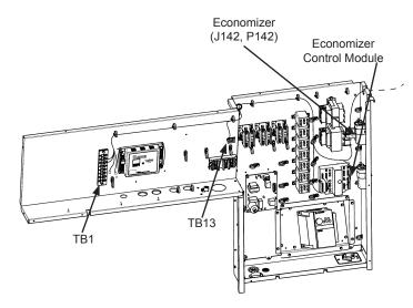
Figure 9 - HVAC Control Box
