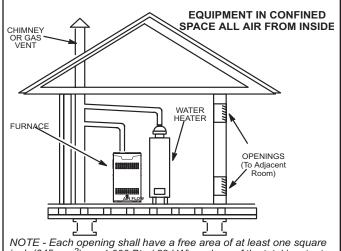
inch (645 mm²) per 1,000 Btu (.29 kW) per hour of the total input rating of all equipment in the enclosure, but not less than 100 square inches (64516 mm²).
