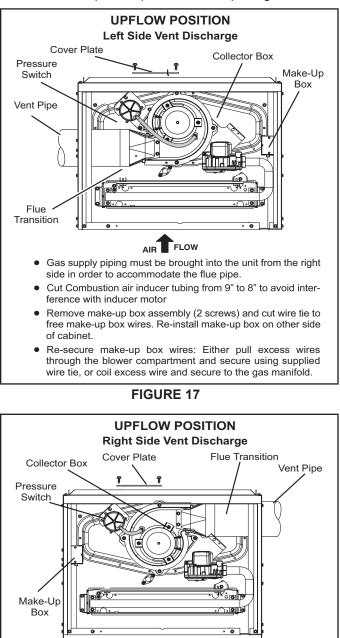
FLOW Cut combustion air inducer tubing from 9" to 5" to avoid interference with inducer motor
