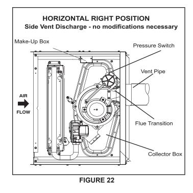
The ML180UHV series units are classified as fan-assisted Category I furnaces when vertically vented according to the latest edition of National Fuel Gas Code (NFPA 54 / ANSI Z223.1) in the USA. A fan-assisted Category I furnace is an appliance equipped with an integral mechanical means to either draw or force combustion products through the combustion chamber and/or heat exchanger. The ML180UHV is not approved for use with horizontal venting.
