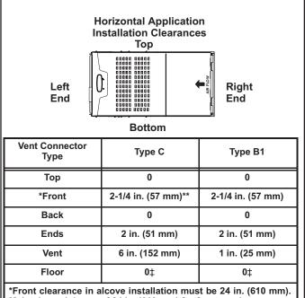
Maintain a minimum of 24 in. (610 mm) for front service access. \*\* 4-1/2 in. if singlewall vent pipe is used.
