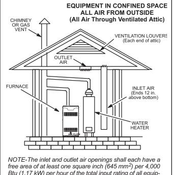
Btu (1.17 kW) per hour of the total input rating of all equipment in the enclosure.
