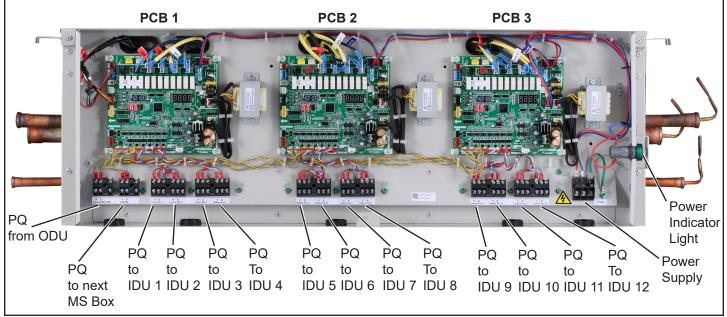
Figure 13 Typical Electrical Control Box (V8MSBB12-3P Shown)
