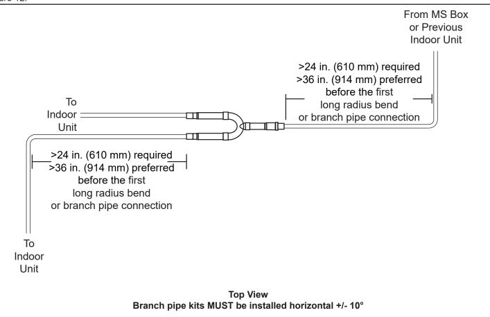
**NOTE -** A maximum of five indoor units can be connected to one port on the mode selection box. The combined maximum capacity of all indoor units connected to one port on a mode selection box must not exceed 54,000 Btus. For larger capacity indoor units, combine two ports using branch joint kit V81DBP06 and the instructions in this manual.
