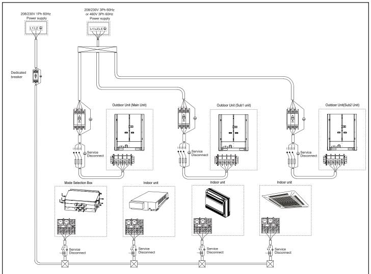
Figure 14. Typical Power Wiring Diagram (VRF Heat Recovery System Shown)
