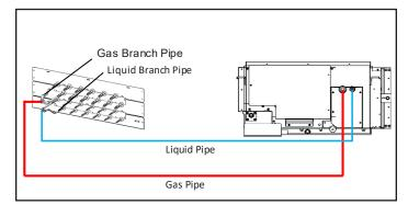
Figure 5. Connect to Indoor Unit Larger than 054k
