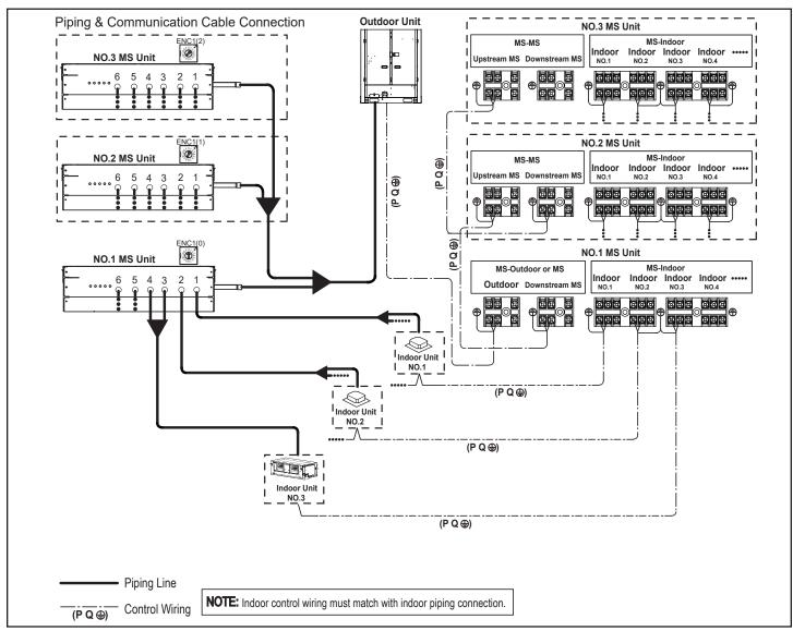
Figure 18. Piping & Communication Cable Routing to Other MS Box on the Same Refrigeration Circuit
