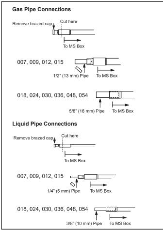
Figure 3. Connect to Indoor Unit 054k and Smaller
