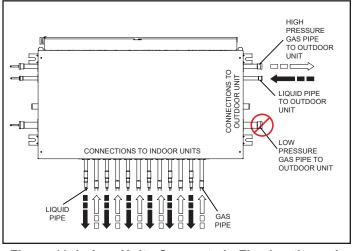
Figure 11. Indoor Units Connected - Flowing through Low Pressure Liquid Line
