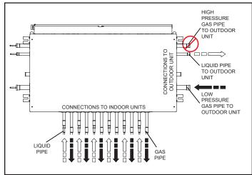
Figure 9. Indoor Units Connected - Flowing through Low Pressure Gas (Suction) Line
