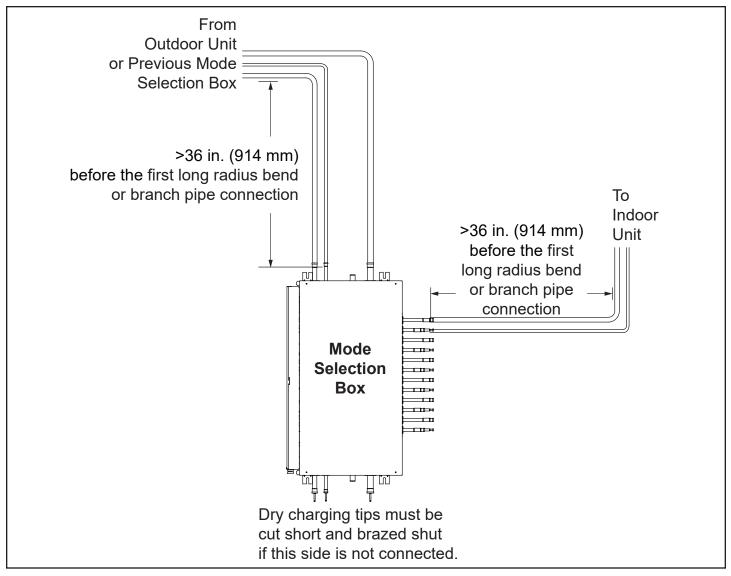
Figure 6. Mode Selection Box Piping
