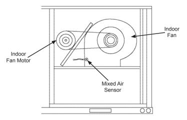
Figure 8A - Mixed Air Sensor Location
