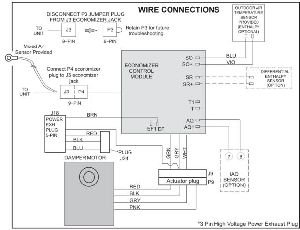
Figure 7 - Wiring Detail
