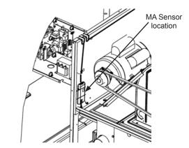
Figure 7 - Mixed Air Sensor Installation
