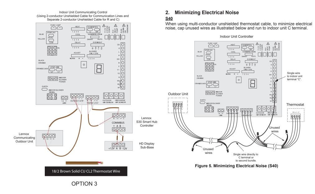
Figure 4. Lennox Communicating System Wiring Connections using Separate Unshielded Cable
