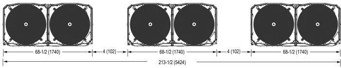
**NOTE** - All the outdoor units manifolded together should be installed at the same elevation.
