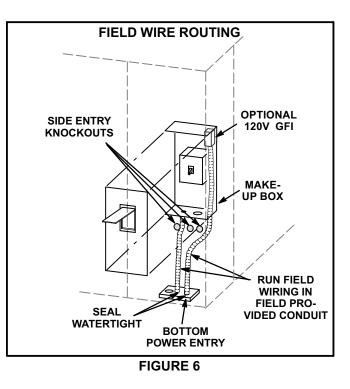
IMPORTANT - Unless field thermostat wires are rated for maximum unit voltage, they must be routed away from line voltage wiring. Use wire ties located in control area to secure thermostat cable.
