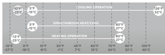
Lennox VRF works in heating mode down to a temperature of \* Extended cooling operation requires accessory low ambient cooling kit -22°F, and cools in temperatures up to 122°F.
