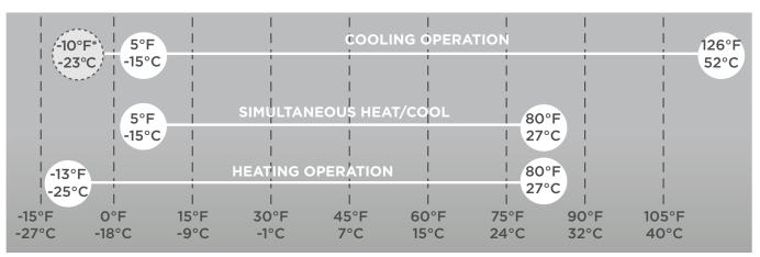
Lennox VRF works in heating mode down to a temperature of -13°F (-25°C), and cools in temperatures up to 126°F (52°C).
