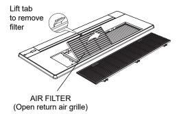
The V22B and V33B filters are accessed through the return air grille as shown in these illustrations.
