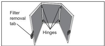
Figure 5. Foldable Factory-Supplied Return Air Filter
