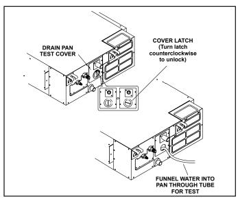
Figure 20. Condensate Drain Test
