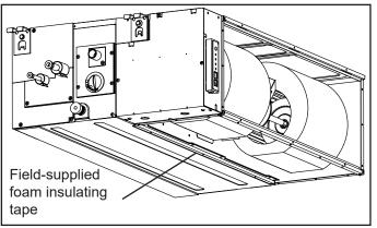
Figure 11. Apply Foam Insulating Tape
