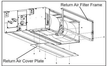
Figure 10. Remove Filter, Filter Frame and Return Air Cover Plate from Existing Location
