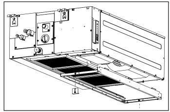
Figure 12. Re-install Filter Frame and Return Air Cover Plate
