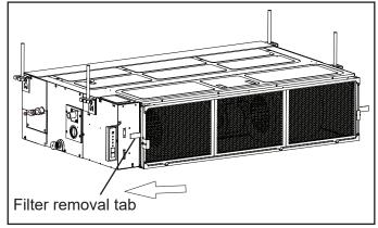
Figure 8. Slide Out Filter
