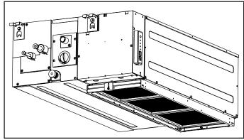
Figure 14. Relocate Return Air Filter Complete
