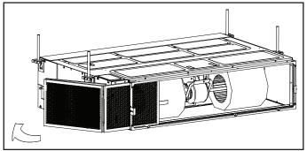
Figure 9. Filter Partially Removed
