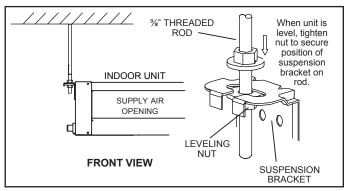
Figure 3. Suspension Hardware
