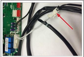
Figure 27. Identify White Plug into Black Wire
