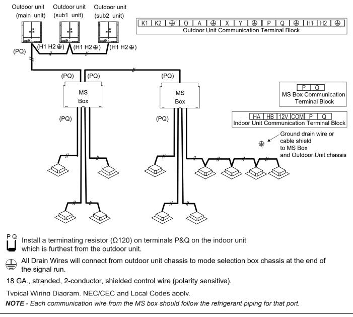
Figure 22. Typical Communication Wiring Diagram (VRF Heat Recovery System)
