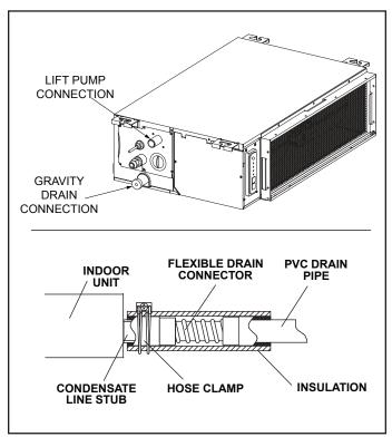
Figure 16. Condensate Drain Connection
