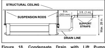
Figure 18. Condensate Drain with Lift Pump Single Unit
