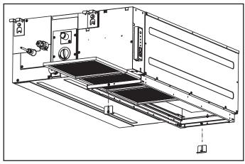
Figure 13. Re-install Filter using Clips
