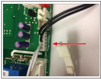
Figure 26. Identify T1 Sensor Connection on PCB
