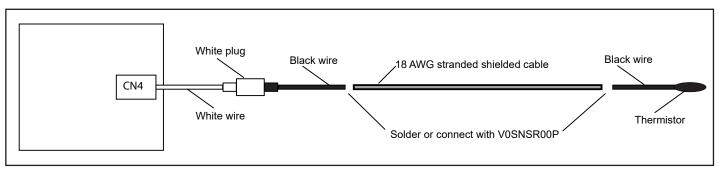
Figure 31. Typical Wiring Connections
