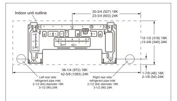
Figure 7. 18K and 24K Indoor Unit Wall Plate Dimensions - Inches (mm)
