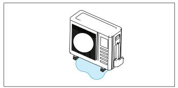
Figure 23. Avoid Defrost Water Ice Hazard
