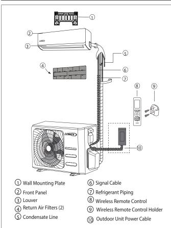
Figure 1. Typical System Shown
