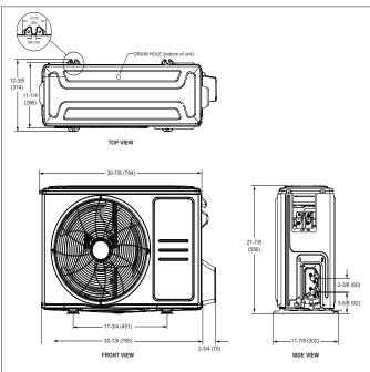
Figure 2. 9K and 12K Outdoor Unit Dimensions - Inches (mm)
