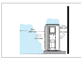
Figure 22. Outdoor Unit Air Flow Obstructed by Snow
