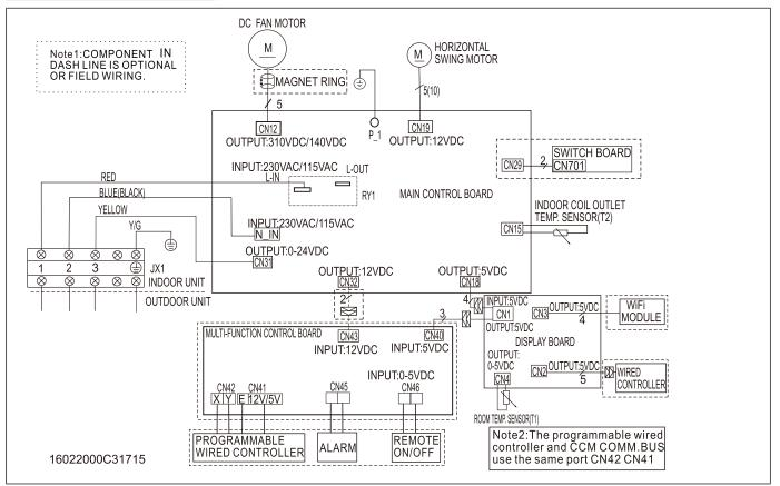
Figure 34. MWHB 09K,12K, and 18K - 115V and 208/230VAC Indoor Unit Wiring Diagram
