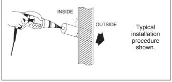
Figure 12. Boring Hole for Wall Sleeve
