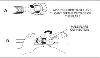
Figure 28. Making Connections (Male to Female Connection)
