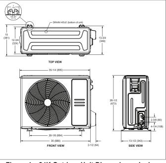
Figure 4. 24K Outdoor Unit Dimensions - Inches (mm)
