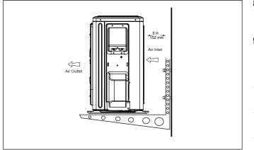
Figure 26. Securing Outdoor Unit to Brackets
