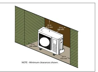
Figure 20. Unit installed in Alcove
