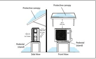
Figure 18. Outdoor Unit on Pedestal and Protective Canopy
