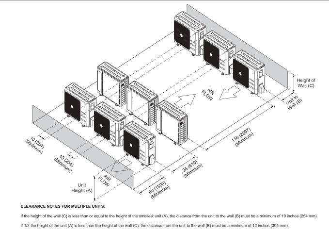
If the height of the wall (C) is greater than the height of the unit (A), the distance from the unit to the wall (B) must be a minimum of 20 inches (508 mm).
