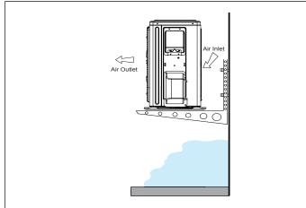
Figure 21. Outdoor Unit on Brackets above Snow Line
