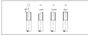
Figure 27. Cutting Piping
