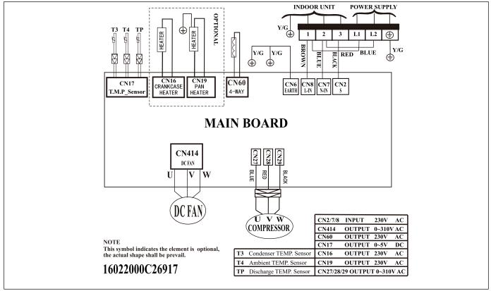
Figure 38. MHB 24K - 208/230VAC Outdoor Unit Wiring Diagram
