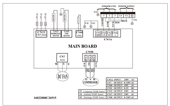
Figure 37. 09K, 12K and 18K - 208/230VAC Outdoor Unit Wiring Diagram
