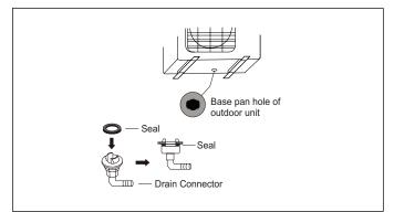
Figure 16. Installing Drain Connector and Seal
