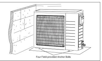
Figure 24. Securing Outdoor Unit to Slab
