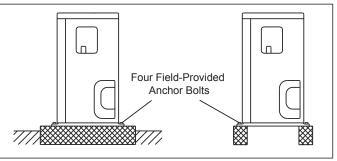
Figure 25. Securing Outdoor Unit to Rails
