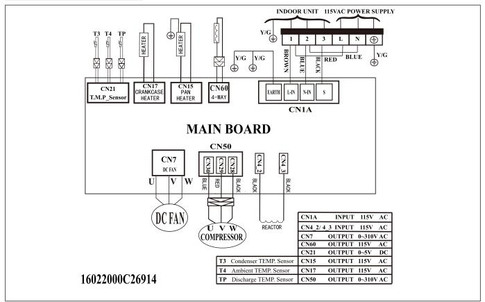
Figure 36. MHB 9K and 12K - 115VAC Outdoor Unit Wiring Diagram
