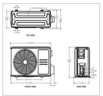
Figure 3. 18K Outdoor Unit Dimensions - Inches (mm)
