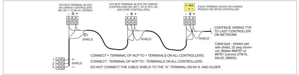
Figure 12. L Connection<sup>®</sup> Network Daisy-Chain Communication Wiring
