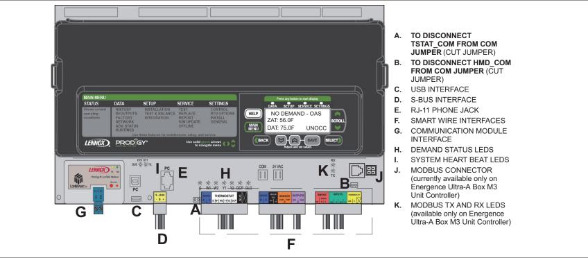
Figure 1. M3 Unit Controller Interfaces and LEDs Locations
