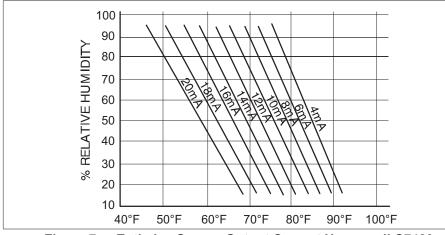
Figure 7. Enthalpy Sensor Output Current Honeywell C7400
