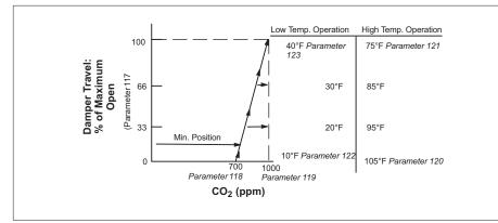
Figure 9. Default Demand Control Ventilation (DCV) Operation
