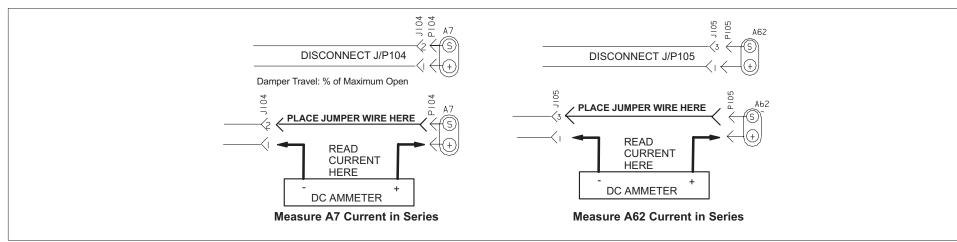
Figure 8. Measure A7 and A62 Current in Series
