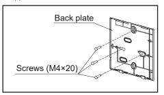
Figure 16. Attach Back Plate to Wall
