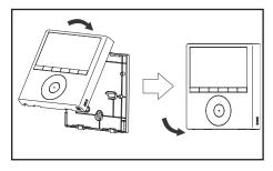
Figure 14. Reattach Controller to Back Plate
