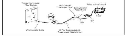
Figure 11. Wiring Connections to MFMA
