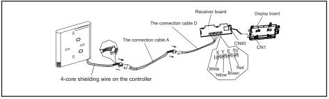
Figure 9. Wiring Connections MWMC, MWCB, and MWHB
