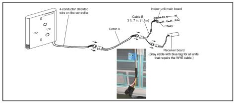
Figure 2. Wiring Connections MMDA/B, MCFA/B, M22A and M33A/B/C
