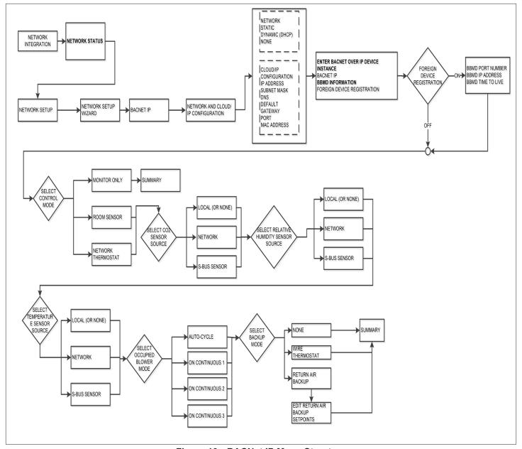
Figure 10. BACNet IP Menu Structure
