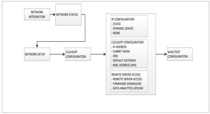
Figure 15. Cloud/IP Configuration Menu Structure
