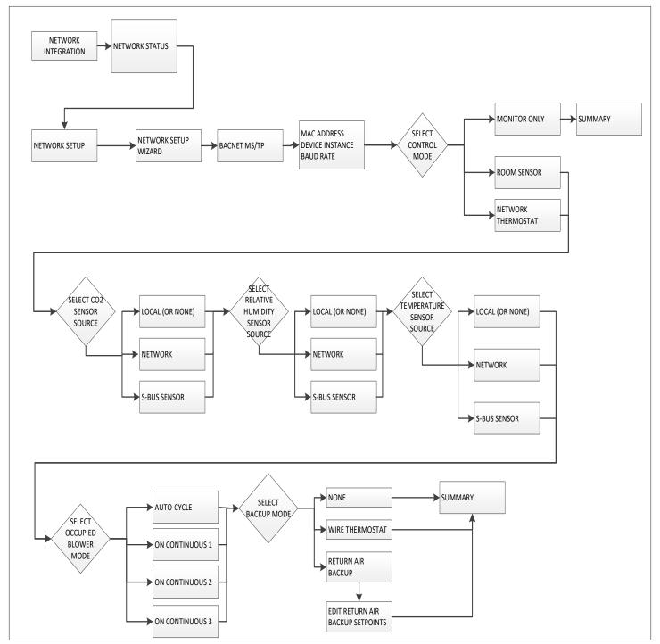
Figure 9. BACNet MS/TP Menu Structure
