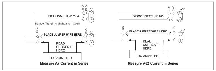
Figure 33. Measure A7 and A62 Current in Series
