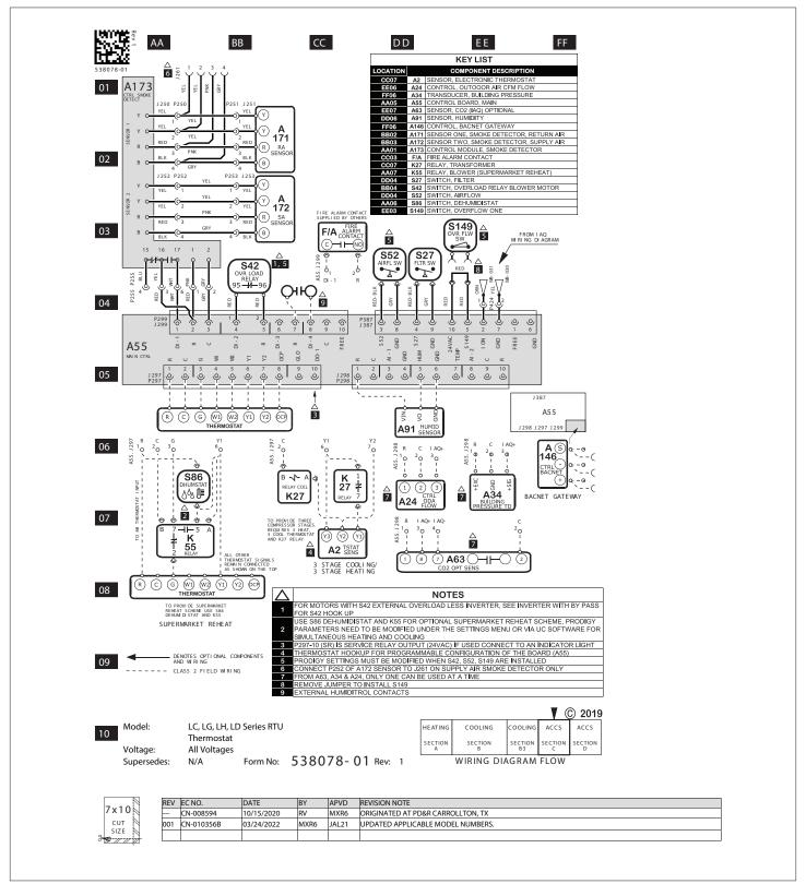
Figure 37. Wiring Diagram
