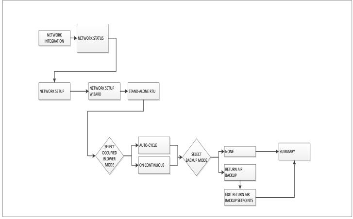
Figure 13. Stand-Alone RTU Menu Structure
