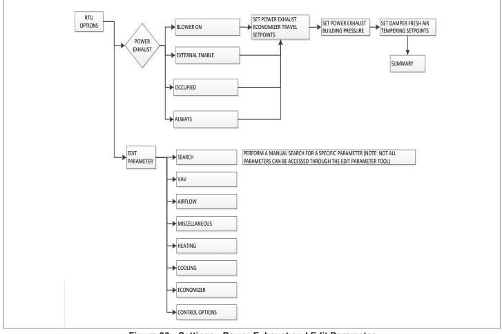
Figure 30. Settings - Power Exhaust and Edit Parameter
