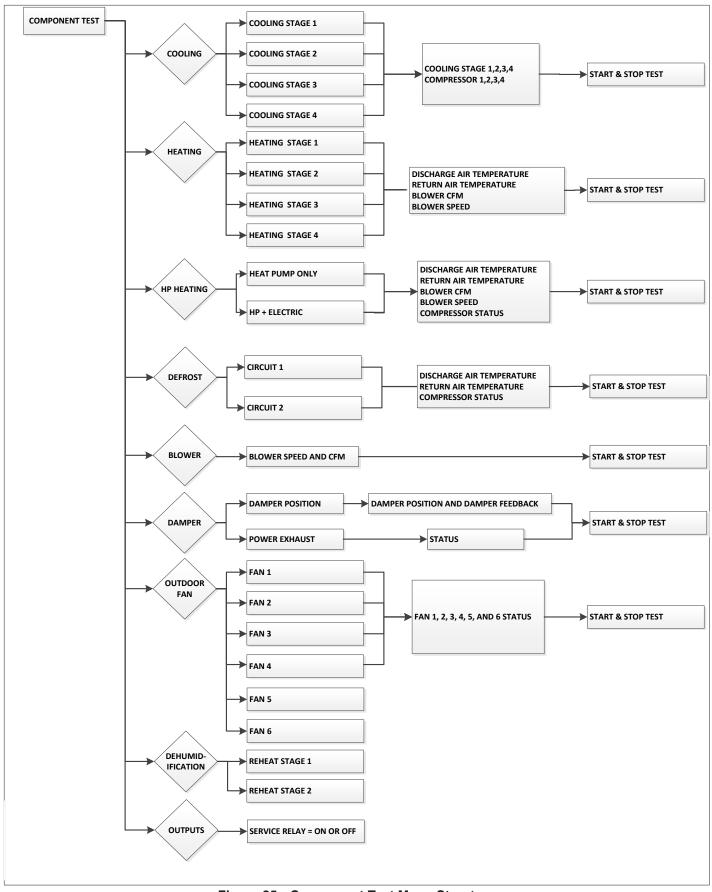
Figure 25. Component Test Menu Structure
