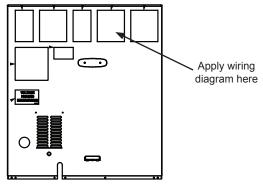
Figure 9 - Label Installation
