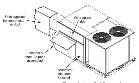
Figure 6 - Installed Economizer
