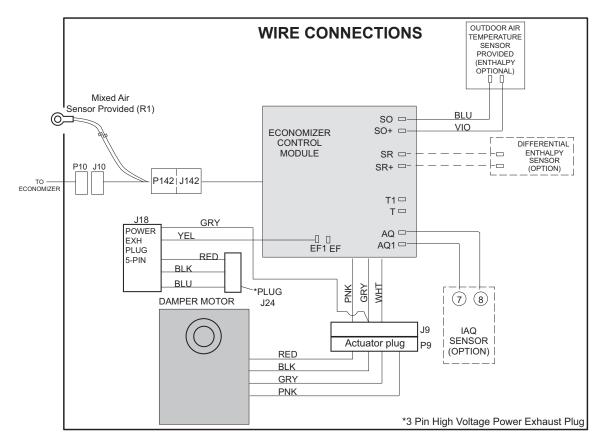
Figure 7 - Wiring Detail
