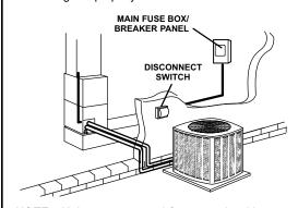
NOTE - Units are approved for use only with copper conductors. Ground unit at disconnect switch or connect to an earth ground.
