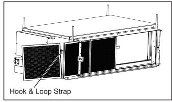
Figure 8. Filter Partially Removed
