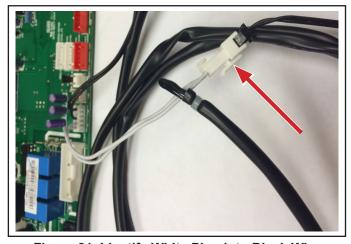
Figure 21. Identify White Plug into Black Wire
