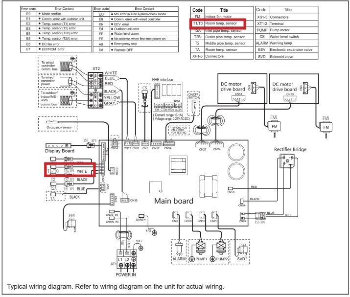
Figure 24. Identify T1 Sensor on Wiring Diagram
