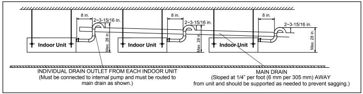
Figure 13. Condensate Drain with Lift Pump Multiple Indoor Units
