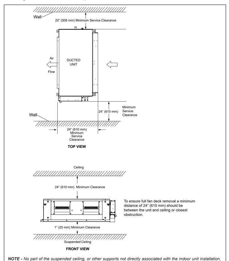
can be fixed to, or touch the indoor unit, in any form. Minimum clearances must be observed at all times.
