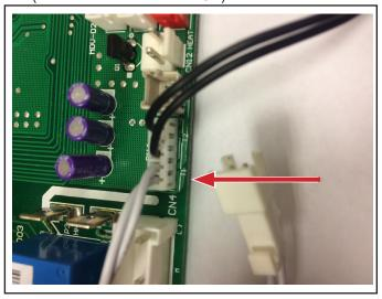
Figure 20. Identify T1 Sensor Connection on PCB
