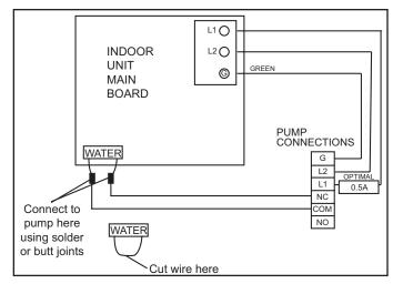
Figure 14. External Water Level Switch Connection
