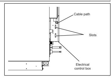
Figure 27. Receiver Mounting Location
