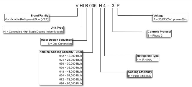
**NOTE -** Only Lennox VRF indoor units will work with Lennox VRF outdoor units and associated mechanical equipment. Lennox Mini Split indoor units are similar in appearance but must not be connected to a Lennox VRF refrigerant circuit. Please refer to model numbers to confirm compatibility. Model numbers for Lennox VRF units start with a "V" and model numbers for Lennox Mini-Splits start with a "M".
