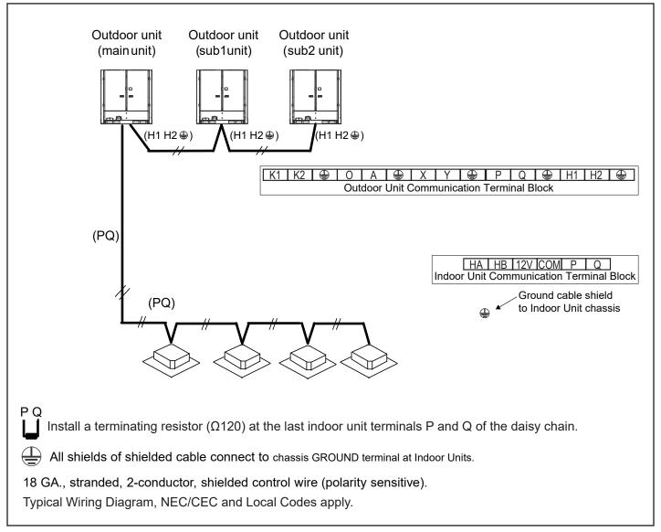
Figure 17. Typical Communication Wiring Diagram (VRF Heat Pump System)
