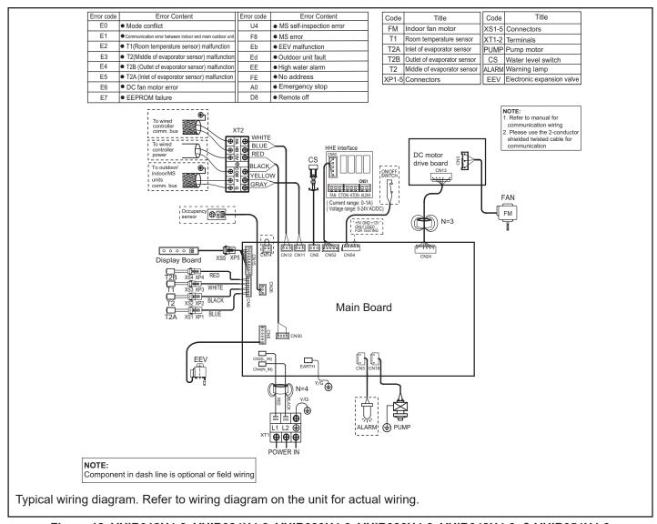
Figure 18. VHIB012H4-3, VHIB024H4-3, VHIB030H4-3, VHIB036H4-3, VHIB048H4-3, & VHIB054H4-3 Typical Wiring Diagram
