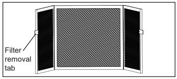
Figure 5. Segmented Factory-Supplied Return Air Filter
