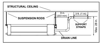
Figure 11. Condensate Drain with Lift Pump Single Unit
