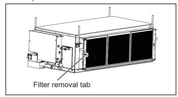
Figure 7. Slide Out Filter
