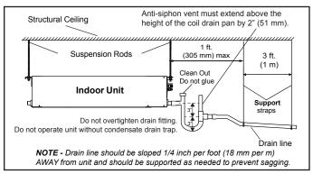
Figure 10. Sloped Condensate Gravity Drain Single Unit
