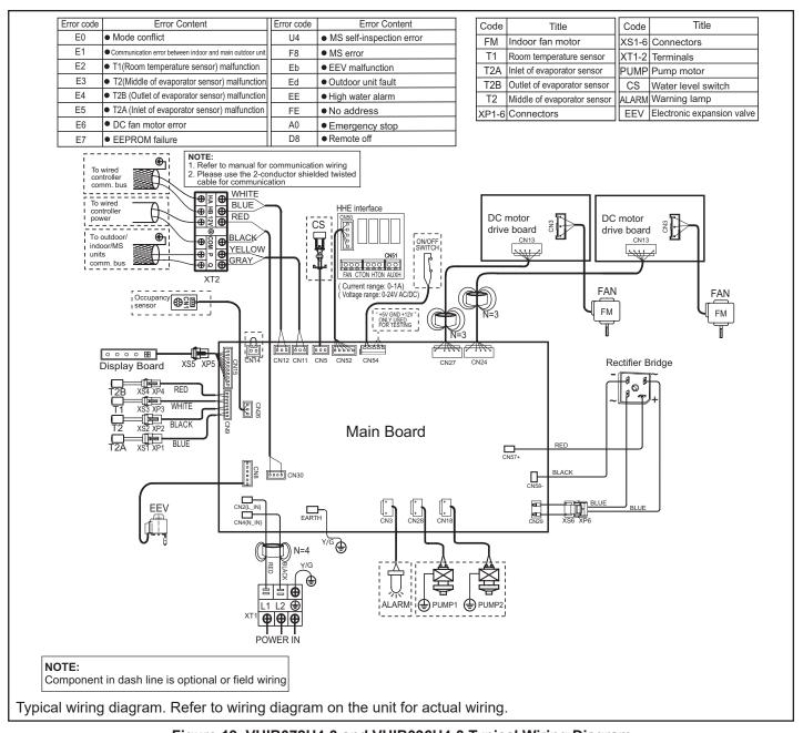
Figure 19. VHIB072H4-3 and VHIB096H4-3 Typical Wiring Diagram
