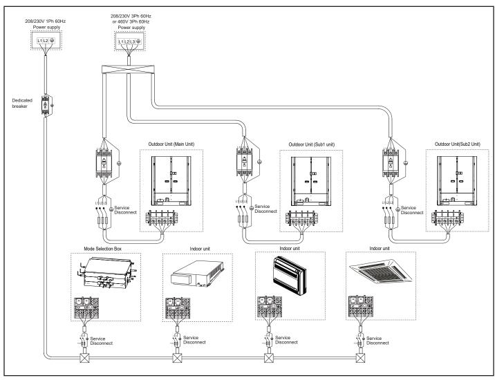
Figure 15. Typical Power Wiring Diagram (VRF Heat Recovery System Shown)
