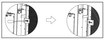
Figure 6. Loosen Filter Retaining Bracket
