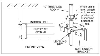
Figure 3. Suspension Hardware
