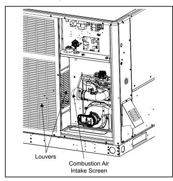
Figure 2. Combustion Intake Screen
