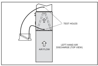
FIGURE 7. Static Pressure Test
