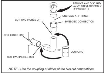
FIGURE 5. CX35 Liquid Line Connections
