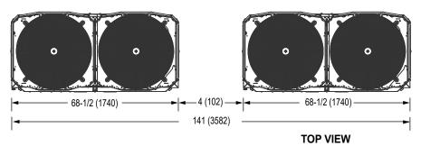
**NOTE** - All the outdoor units manifolded together should be installed at the same elevation.
