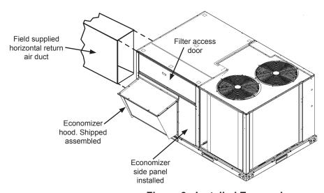
Figure 6 - Installed Economizer
