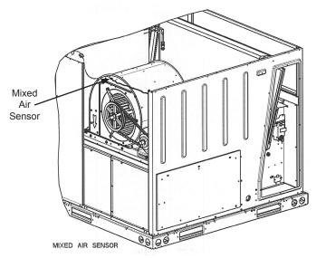
Figure 8 - Mixed Air Sensor Location
