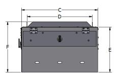
FILTER(S) CAN BE INSERTED FROM SIDE OR BOTTOM. FILTER BOXES 2" STANDARD DEPTH FILTERS.
