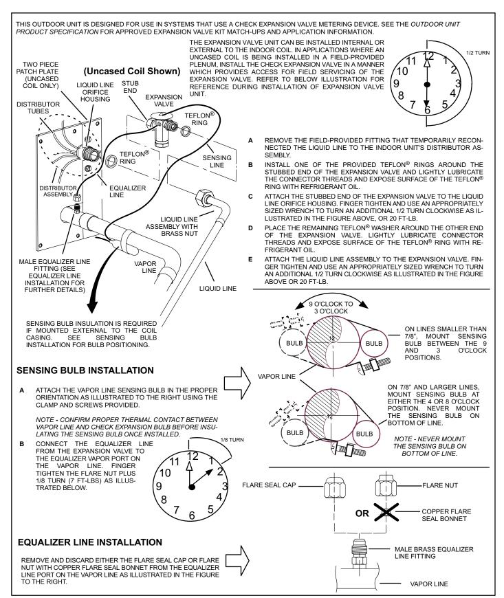
Figure 3. Typical TXV Metering Device Removal and Installation Procedure
