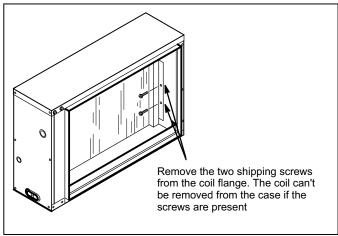
Figure 1. Removing Shipping Screws
