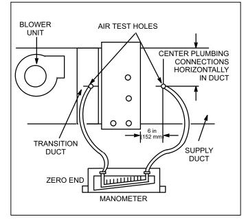
Figure 6. Air Test Hole Locations
