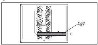
**FIGURE 1. Insulate Suction Line Inside Cabinet**
