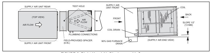
FIGURE 5. Right-Hand Air Discharge with Spacer
