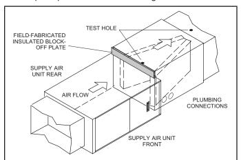
FIGURE 2. D-Width Coil with C-Width Furnace
