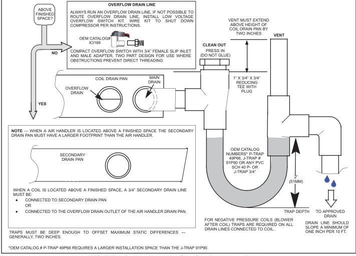
FIGURE 8. Typical Main and Overflow Drain Installations
