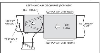
**FIGURE 9. Static Pressure Test**
