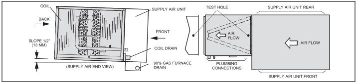
FIGURE 3. Left-Hand Air Discharge
