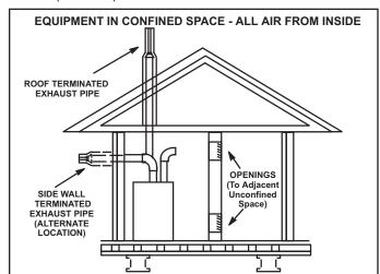
**NOTE** - Each opening shall have a free area of at least one square inch per 1,000 Btu (645mm<sup>2</sup> per .29kW) per hour of the total input rating of all equipment in the enclosure, but not less than 100 square inches (64516mm.<sup>2</sup>).
