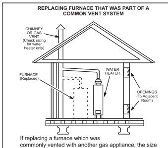
If replacing a furnace which was commonly vented with another gas appliance, the size of the existing vent pipe for that gas appliance must be checked. Without the heat of the original furnace flue products, the existing vent pipe is probably oversized for the single water heater or other appliance. The vent should be checked for proper draw with the remaining appliance.
