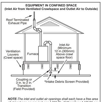
**NOTE**-The inlet and outlet air openings shall each have a free area of at least one square inch per 4,000 Btu (645mm<sup>2</sup> per 1.17kW) per hour of the total input rating of all equipment in the enclosure.
