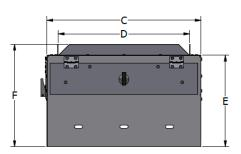
FILTER(S) CAN BE INSERTED FROM SIDE OR BOTTOM. FILTER BOXES 4" STANDARD DEPTH FILTERS.
