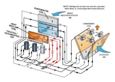
unit will dehumidify and cool all the air entering the unit with the evaporator coils and then warm up the conditioned air using the reheat coils. This will allow the unit to return fully dehumidified air back to the occupied space at a neutral air temperature.
