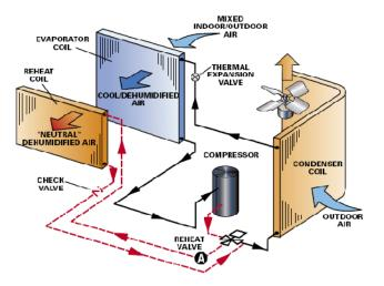
Hot gas (200F or more) exiting compressor increases ability of reheat coil to reheat air up to neutral conditions
