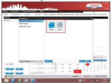
Figure 30. Select Indoor Units to Remove
