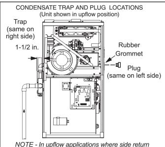
air filter is installed on same side as the condensate trap, filter rack must be installed beyond condensate trap or trap must be re-located to avoid interference.
