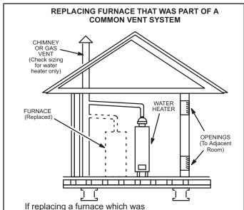
commonly vented with another gas appliance, the size of the existing vent pipe for that gas appliance must be checked. Without the heat of the original furnace flue products, the existing vent pipe is probably oversized for the single water heater or other appliance. The vent should be checked for proper draw with the remaining appliance.
