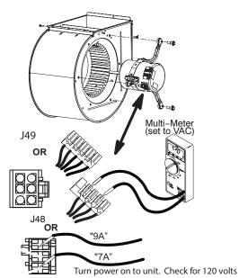
across terminals "L" and "N" or terminals "7A" Test 1 and "9A" of connector J48. If voltage is present continue to test 2. If voltage is not present problem may be upstream of J48. Proceed to test3.
