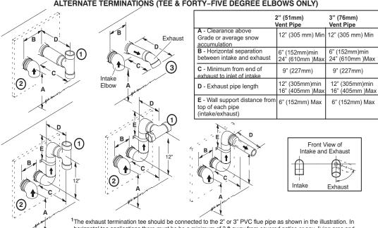
horizontal tee applications there must be be a minimum of 3 ft away from covered patios or any living ares and cannot be within 3 ft of a window. Do not use an accelerator in applications that include an exhaust termination tee. The accelerator is not required.
