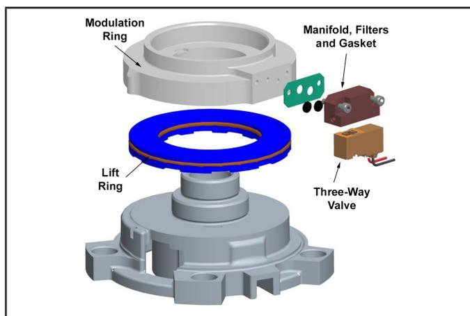
FIGURE 4. Two-Stage Scroll Compressor
