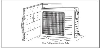
Figure 27. Securing Outdoor Unit to Slab
