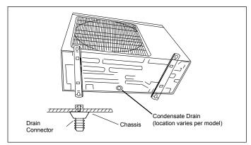
Figure 26. Condensate Drain
