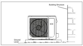
Figure 18. Install Unit Level
