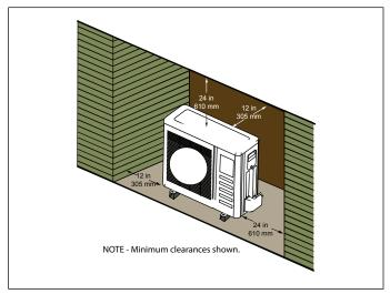
Figure 25. Unit installed in Alcove
