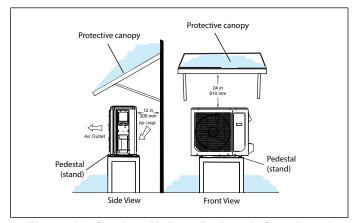
Figure 19. Outdoor Unit on Pedestal (Stand) and Protective Canopy
