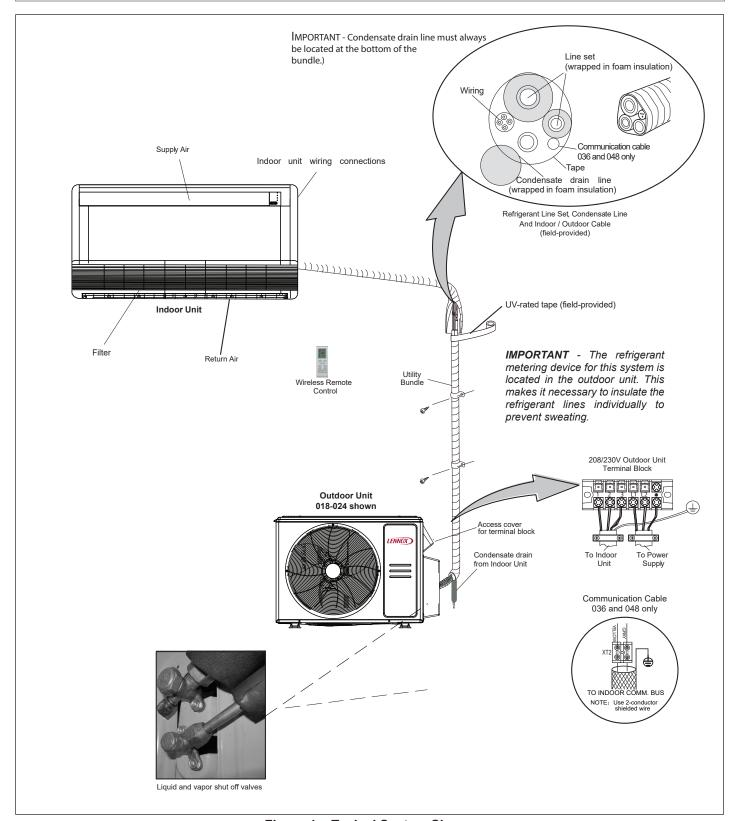
Figure 1. Typical System Shown
