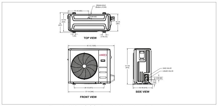
Figure 6. MLB024S4S Outdoor Unit Dimensions - Inches (mm)
