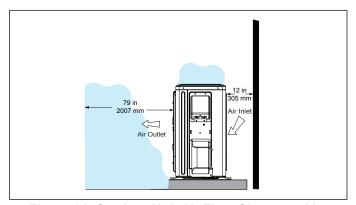
Figure 21. Outdoor Unit Air Flow Obstructed by Snow
