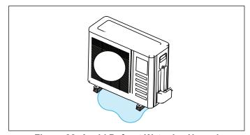
Figure 22. Avoid Defrost Water Ice Hazard
