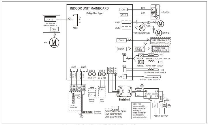
Figure 38. MCFA048S4-\*P Unit Wiring Diagram
