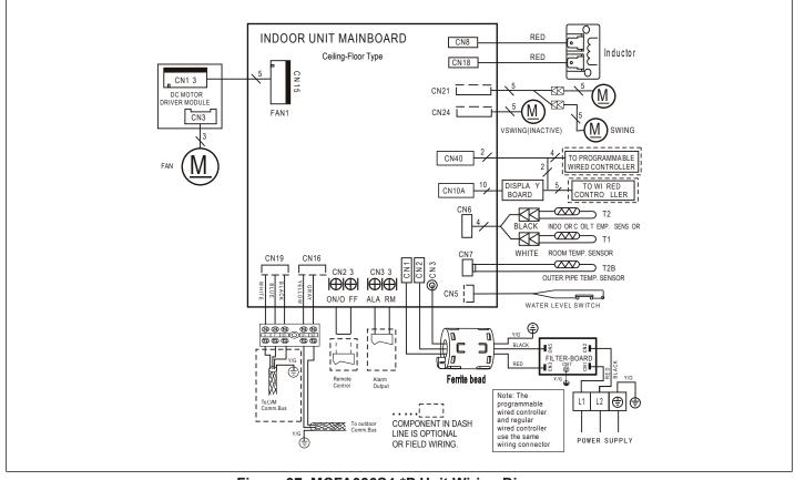
Figure 37. MCFA036S4-\*P Unit Wiring Diagram
