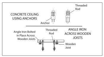
Figure 15. Locate Threaded Rods
