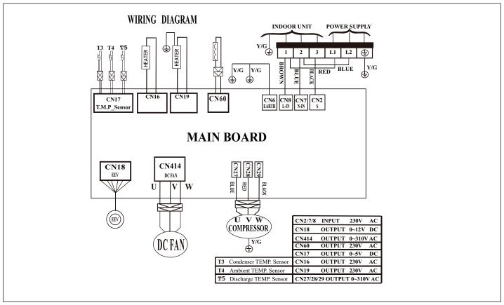
Figure 40. 208/230V MPC024S4S-\*P Outdoor Unit Wiring Diagram
