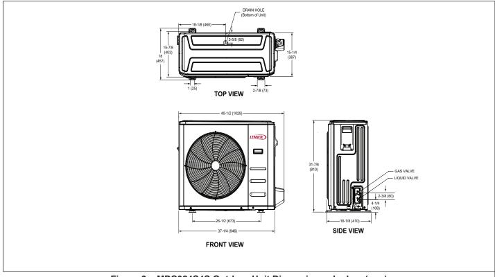
Figure 3. MPC024S4S Outdoor Unit Dimensions - Inches (mm)
