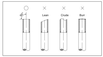
Figure 30. Cutting Pipe
