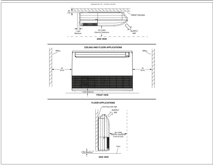
Figure 10. Indoor Unit Clearances - Inches (mm)
