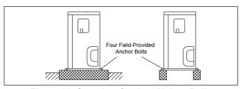
Figure 28. Securing Outdoor Unit to Rails
