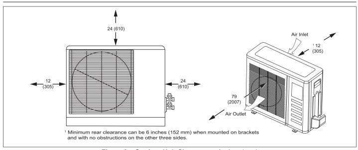
Figure 9. Outdoor Unit Clearances - Inches (mm)
