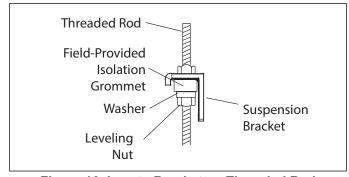
Figure 16. Locate Bracket on Threaded Rod
