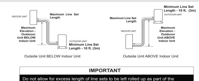
Do not allow for excess length of line sets to be left rolled up as part of the required distance, or in general. This will also cause additional performance issues.
