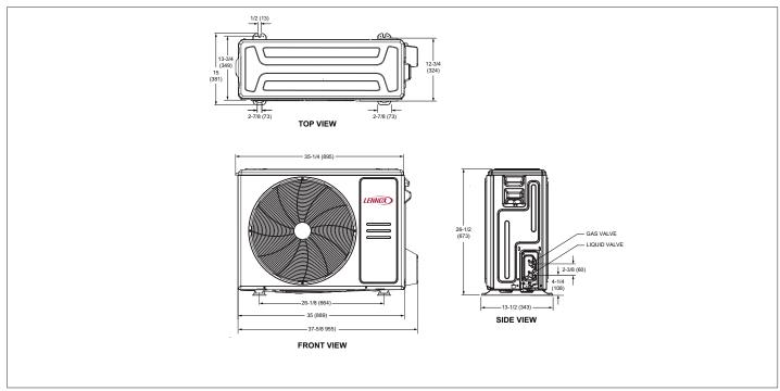
Figure 5. MLB018S4S Outdoor Unit Dimensions - Inches (mm)
