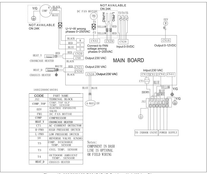
Figure 43. 208/230V MLB024S4S-\*P Outdoor Unit Wiring Diagram
