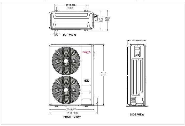
Figure 7. MLB036S4S and MLB048S4S Outdoor Unit Dimensions - Inches (mm)
