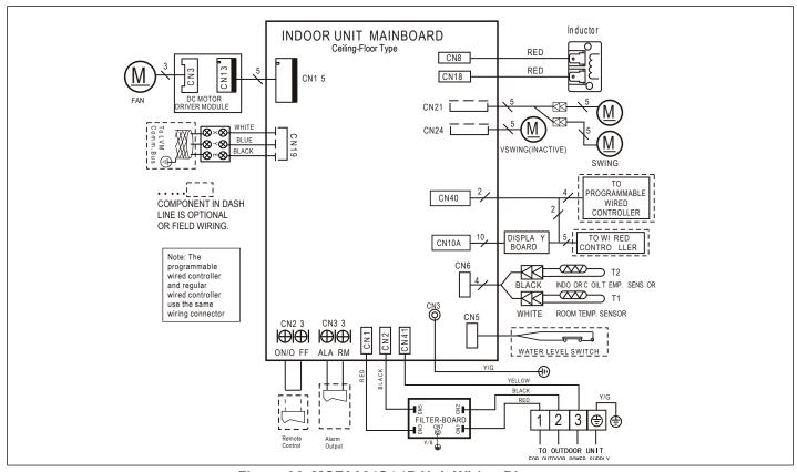
Figure 36. MCFA024S4-\*P Unit Wiring Diagram
