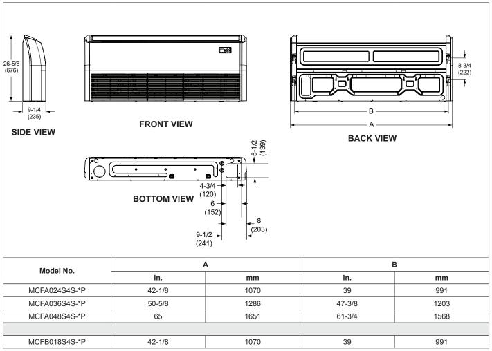
Figure 8. MCFA and MCFB Indoor Unit Dimensions - Inches (mm)
