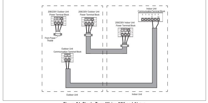
Figure 34. Single-Zone Wiring 36K and Above
