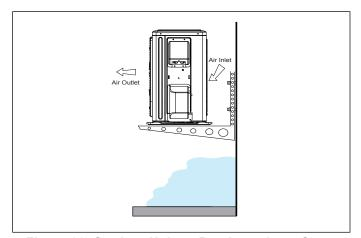
Figure 20. Outdoor Unit on Brackets above Snow Line
