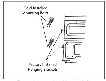
Figure 13. Hang Unit on Mounting Bolts
