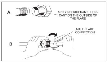
Figure 31. Making Connections (Male to Female Connection)
