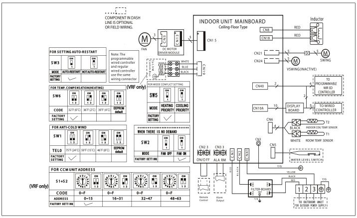
Figure 35. MCFB018S4-\*P Unit Wiring Diagram
