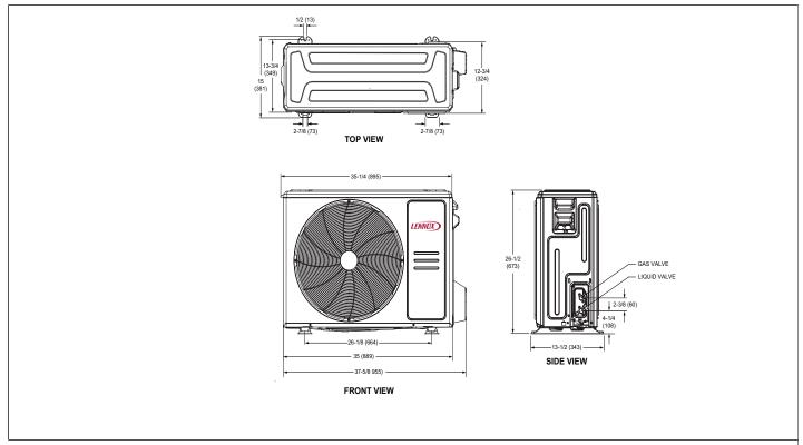
Figure 2. MPC018S4S Outdoor Unit Dimensions - Inches (mm)
