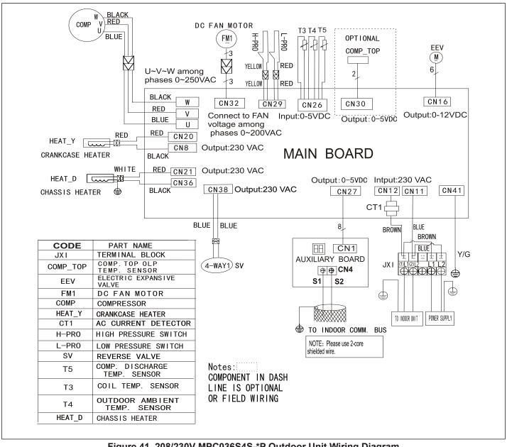
Figure 41. 208/230V MPC036S4S-\*P Outdoor Unit Wiring Diagram
