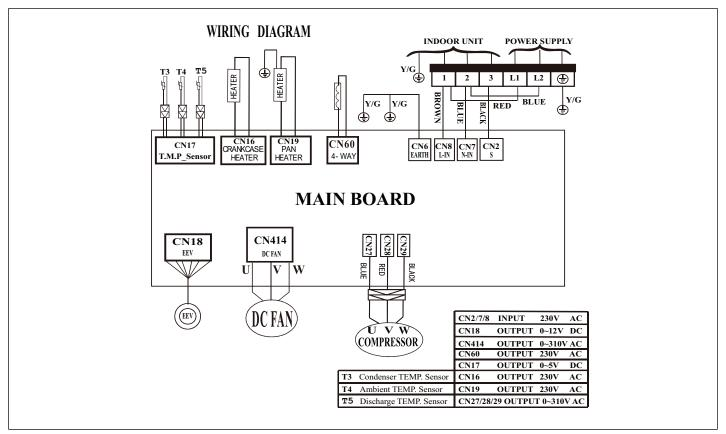
Figure 39. 208/230V MPC018S4S-\*P Outdoor Unit Wiring Diagram
