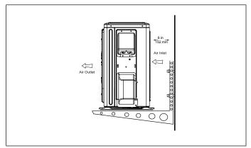
Figure 29. Securing Outdoor Unit to Brackets
