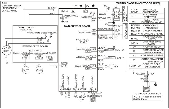
Figure 42. 208/230V MPC048S4S-\*P Outdoor Unit Wiring Diagram
