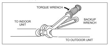
Figure 32. Tighten Flare Nut
