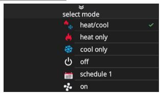
Touch current operating mode on home screen under temperature display to access **Select Mode** screen.
