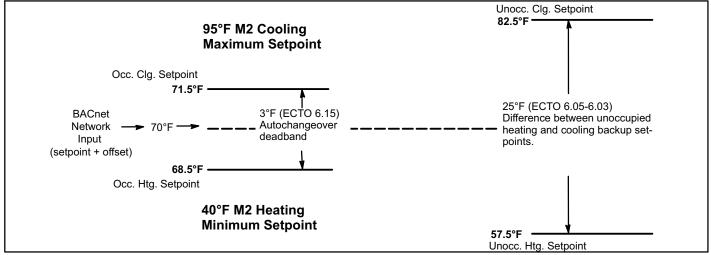
Figure 2. M2 Default Setpoint Example (Zone Sensor Installed)
