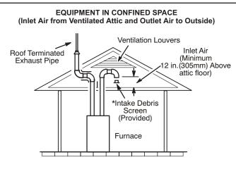
**NOTE**-The inlet and outlet air openings shall each have a free area of at least one square inch per 4,000 Btu (645mm<sup>2</sup> per 1.17kW) per hour of the total input rating of all equipment in the enclosure.
