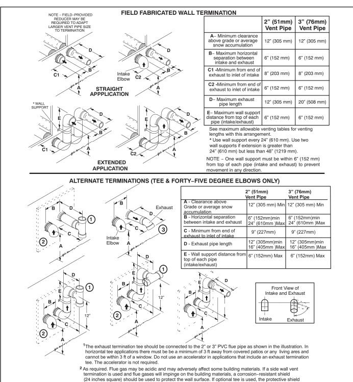
(24 incres square) should be used to protect the waii surface. In optional teels used, the protective sheet is recommended. The shield should be constructed using wood, sheet metal or other suitable material. All seams, joints, cracks, etc. in affected area, should be sealed using an appropriate sealant. <sup>3</sup> Exhaust pipe 45° elbow can be rotated to the side away from the combustion air inlet to direct exhaust
