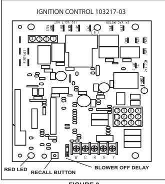
FIGURE 3 Electronic Ignition (FIGURE 13)
