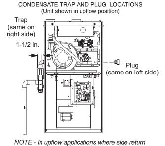
NOTE - In upflow applications where side return air filter is installed on same side as the condensate trap, filter rack must be installed beyond condensate trap or trap must be re-located to avoid interference.
