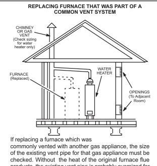
of the existing vent pipe for that gas appliance must be checked. Without the heat of the original furnace flue products, the existing vent pipe is probably oversized for the single water heater or other appliance. The vent should be checked for proper draw with the remaining appliance.
