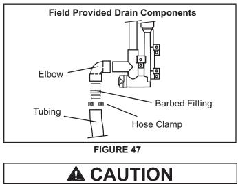
Do not use copper tubing or existing copper condensate lines for drain line.
