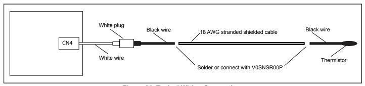
**Figure 25. Typical Wiring Connections**
