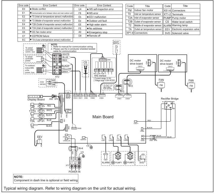
Figure 19. VOSB072H4-3 and VOSB096H4-3 Typical Wiring Diagram
