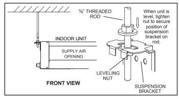
Figure 3. Suspension Hardware
