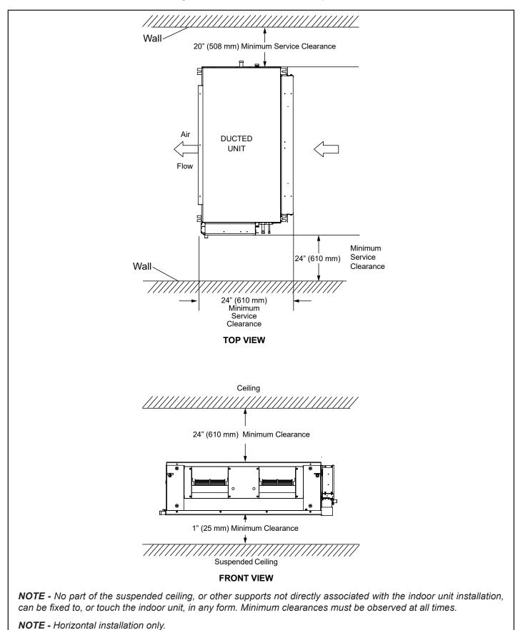
**Figure 1. Minimum Installation Clearances**
