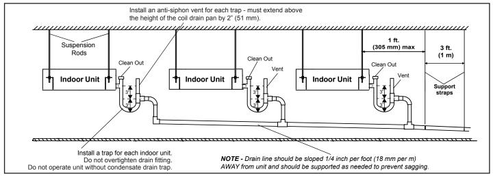
Figure 12. Sloped Condensate Gravity Drain Multiple Indoor Units
