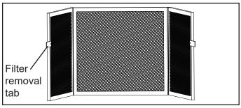
Figure 5. Segmented Factory-Supplied Return Air Filter
