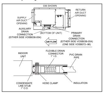
Figure 9. Condensate Drain Connection
