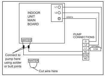
Figure 14. External Water Level Switch Connection
