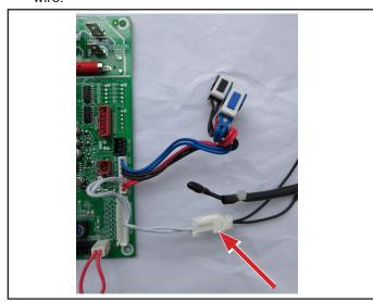
Figure 21. Identify White Plug into Black Wire
