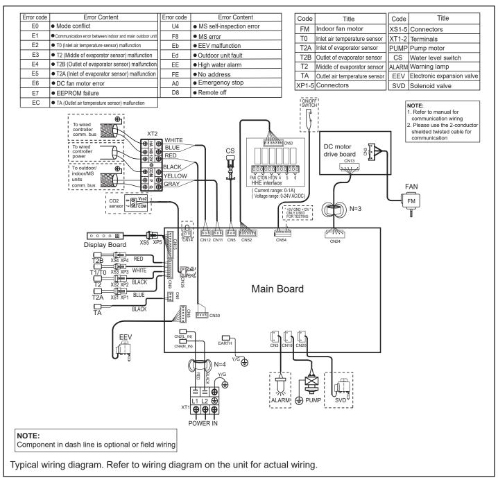
Figure 18. VOSB036H4-3, VOSB048H4-3, & VOSB054H4-3 Typical Wiring Diagram
