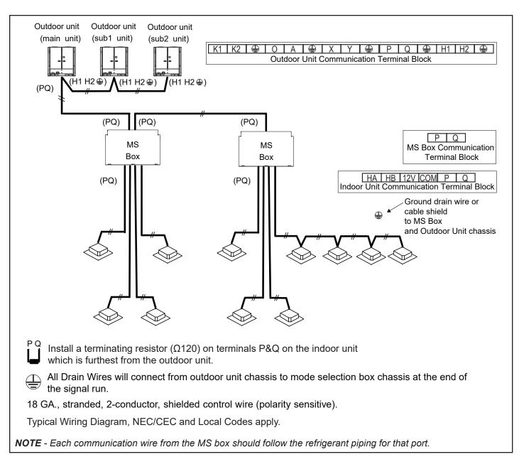
Figure 16. Typical Communication Wiring Diagram (VRF Heat Recovery System)
