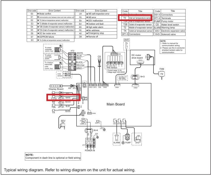
Figure 24. Identify T0 Sensor on Wiring Diagram
