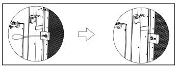
Figure 6. Loosen Filter Retaining Bracket
