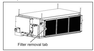
Figure 7. Slide Out Filter
