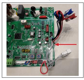
Figure 20. Identify T0 Sensor Connection on PCB
