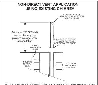
NOTE - Do not discharge exhaust gases directly into any chimney or vent stack. If vertical discharge through an existing unused chimney or stack is required, insert piping inside chimney until the pipe open end is above top of chimney and terminate as illustrated. In any exterior portion of chimney, the exhaust vent must be insulated.
