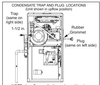
NOTE - In upflow applications where side return air filter is installed on same side as the condensate trap, filter rack must be installed beyond condensate trap or trap must be re-located to avoid interference.
