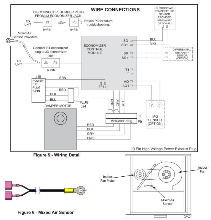
Figure 6A - Mixed Air Sensor Location
