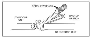
Figure 36. Tighten Flare Nut
