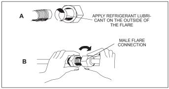
Figure 35. Making Connections (Male to Female Connection)
