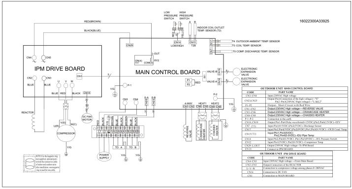
Figure 45. 208/230V MLB018S4S-\*P Outdoor Unit Wiring Diagram
