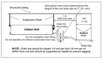
Figure 19. Slope Condensate Drain
