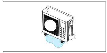
Figure 26. Avoid Defrost Water Ice Hazard
