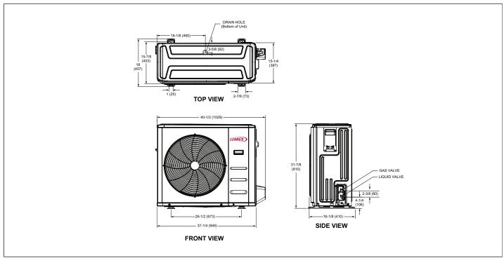
Figure 5. MPC036S4S Outdoor Unit Dimensions - Inches (mm)
