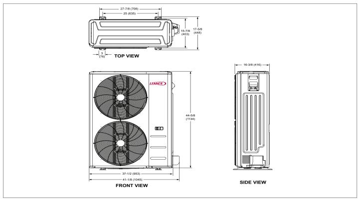
Figure 10. Outdoor Unit Dimensions (MLB036S4S-\*P, MLB048S4S-\*P) - Inches (mm)
