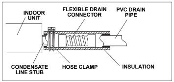
Figure 18. Condensate Gravity Drain Option
