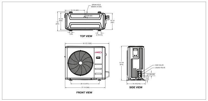
Figure 9. MLB024S4S Outdoor Unit Dimensions - Inches (mm)
