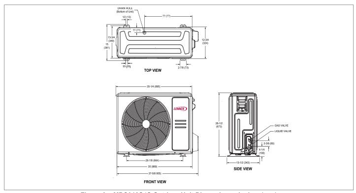
Figure 3. MPC018S4S Outdoor Unit Dimensions - Inches (mm)
