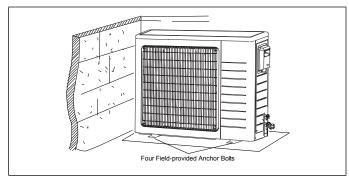
Figure 31. Securing Outdoor Unit to Slab
