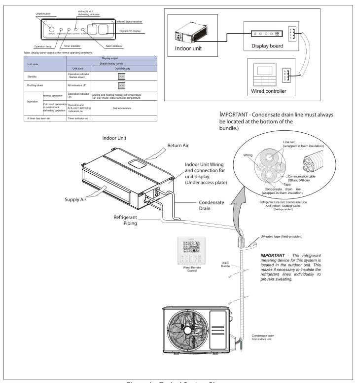
Figure 1. Typical System Shown
