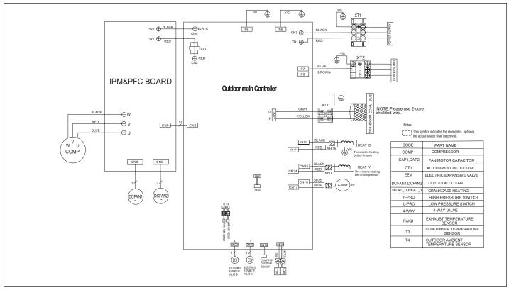
Figure 47. 208/230V MLB036S4S-\*P and MLB048S4S-\*P Outdoor Unit Wiring Diagram
