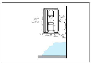
Figure 24. Outdoor Unit on Brackets above Snow Line
