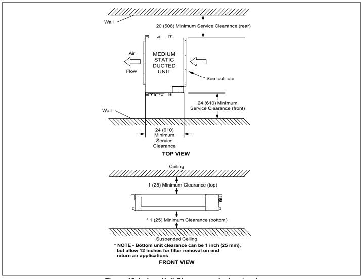
Figure 13. Indoor Unit Clearances - Inches (mm)
