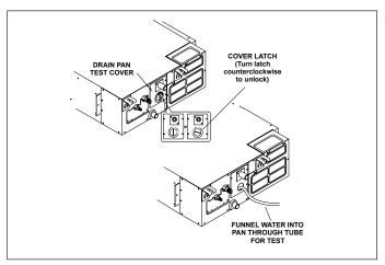
Figure 21. Condensate Drain Test
