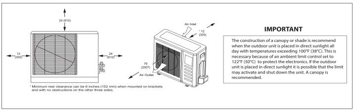
Figure 12. Outdoor Unit Clearances - Inches (mm)
