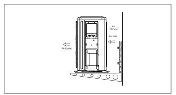
Figure 33. Securing Outdoor Unit to Brackets
