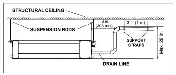
Figure 20. Condensate Drain with Factory Condensate Pump
