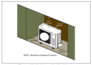
Figure 29. Unit installed in Alcove
