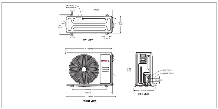
Figure 8. MLB018S4S Outdoor Unit Dimensions - Inches (mm)
