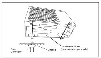
Figure 30. Condensate Drain
