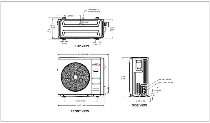
Figure 4. MPC024S4S Outdoor Unit Dimensions - Inches (mm)
