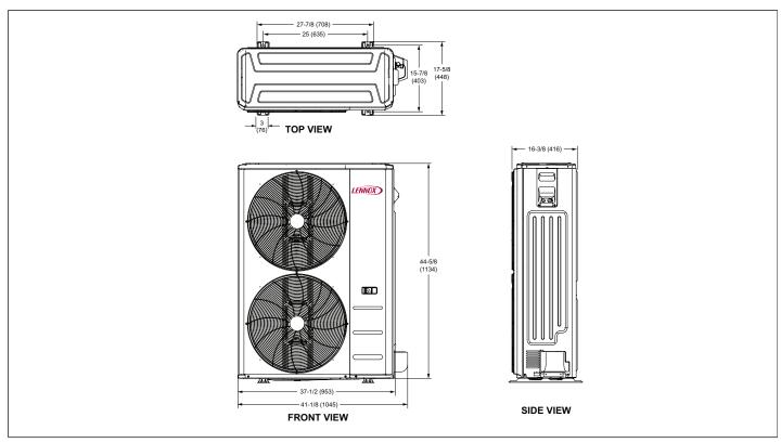
Figure 6. MPC048S4S Outdoor Unit Dimensions - Inches (mm)
