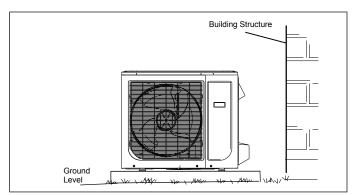
Figure 22. Install Unit Level
