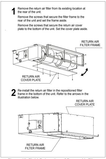
Figure 17. Field-Relocation of Return Air Filter (Typical) - Bottom Return Air
