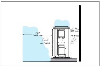
Figure 25. Outdoor Unit Air Flow Obstructed by Snow
