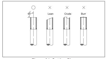
Figure 34. Cutting Pipe
