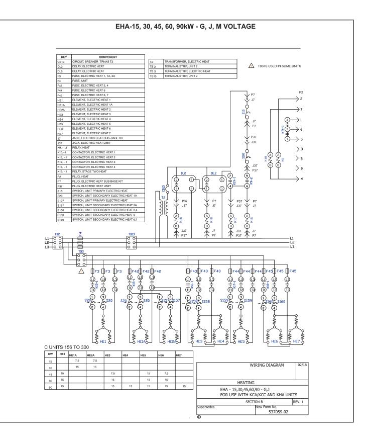
**NOTE:** This sequence of operation is for all Electric Heat *kW* ratings Y, G, J and M voltages.
