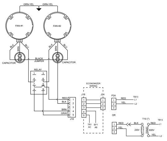
Figure 8 - Wiring Diagram for 230v 1PH
