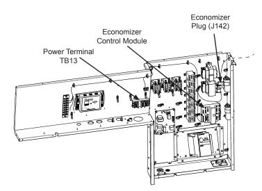
Figure 3 - HVAC Control Box
