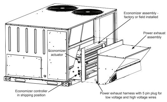
Figure 5 - Power Exhaust Installation
