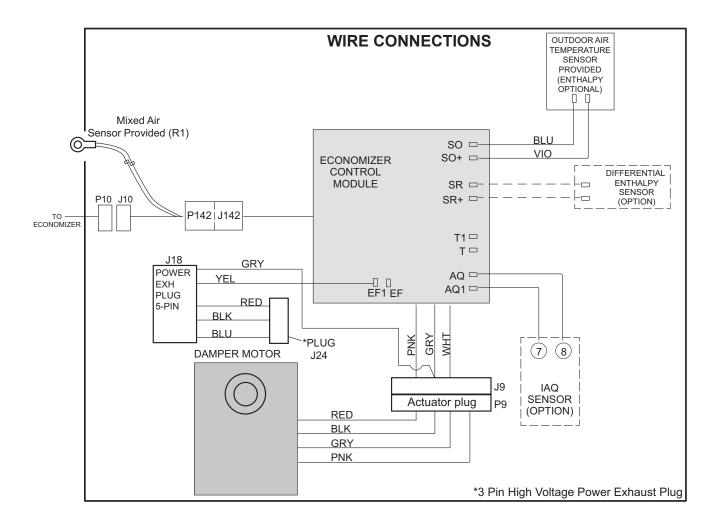
Figure 5 - Wiring Detail
