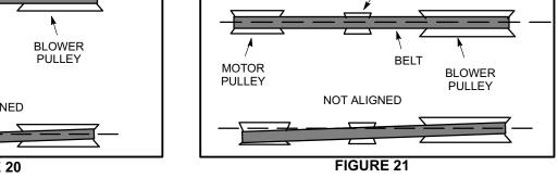
**PULLEY ALIGNMENT - WITH TENSIONER**
