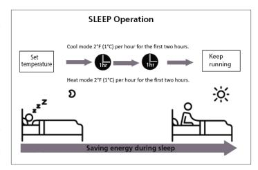
NOTE: While in sleep mode these features (active clean, silence feature, breeze away function, refrigerant leakage detection and Eco features) are not available.
